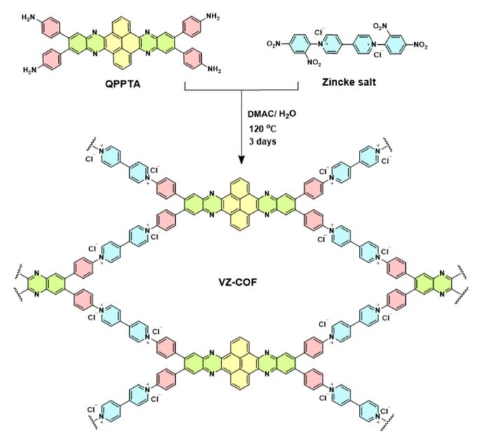
Scheme 1 Synthesis of VZ-COF using the Zincke reaction.
