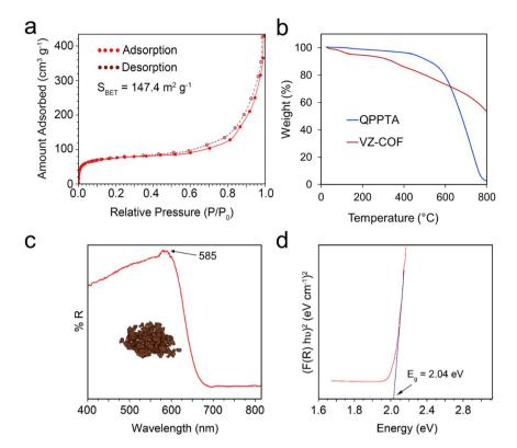
Fig. 4 (a)  $N_2$  adsorption and desorption isotherms of VZ-COF. (b) TGA thermograms of VZ-COF and QPPTA. (c) UV-vis DRS spectrum of VZ-COF. (d) The optical band gap value of VZ-COF, obtained from the Kubelka–Munk-transformed reflectance spectra.
