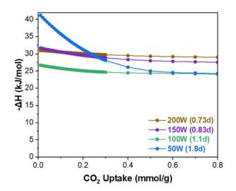
Fig. 6 CO<sub>2</sub> isosteric heat of adsorption of the MW-assisted synthesized UiO-66 with varying MW power.
