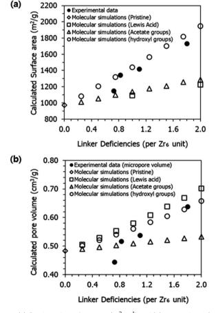
Fig. 9 (a) Gravimetric surface area ( $m^2$   $g^{-1}$ ) and (b) pore volume ( $cm^3$   $g^{-1}$ ) for pristine and defective UiO-66 structures with various terminations: experimental data and molecular simulations. The positions of the terminated groups were optimized using geometry optimization with the UFF force field.
