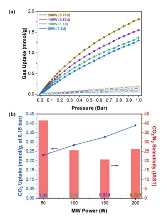
Fig. 5 (a) CO<sub>2</sub> and N<sub>2</sub> pure gas isotherms at 30 °C of UiO-66 synthesized under MW irradiation with varying MW power and (b) IAST  $CO_2$  uptake (line) at 0.15 bar and  $CO_2/N_2$  selectivity (bar) as a function of MW power.
