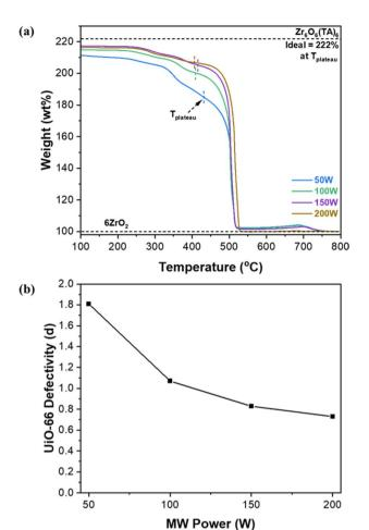
Fig. 3 (a) TGA thermograms of UiO-66 synthesized under MW irradiation with varying MW power and (b) defectivity (d) of MW-assisted synthesized UiO-66 as a function of MW-radiation power.
