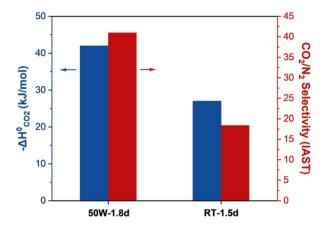
Fig. 7 Comparison of the MW (50 W-1.8d) and TH (RT-1.5d) samples with the highest defectivity respectively: CO2 heat of adsorption at zero CO<sub>2</sub> coverage (blue bar) and CO<sub>2</sub>/N<sub>2</sub> IAST selectivity (red bar).
