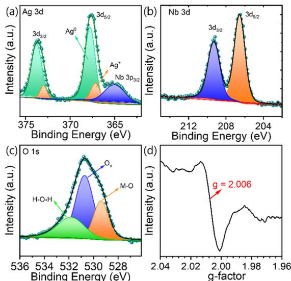
Fig. 2 High-resolution spectra of (a) Ag 3d, (b) Nb 3d, and (c) O 1s. (d) EPR data of AgNbO<sub>3</sub>.
