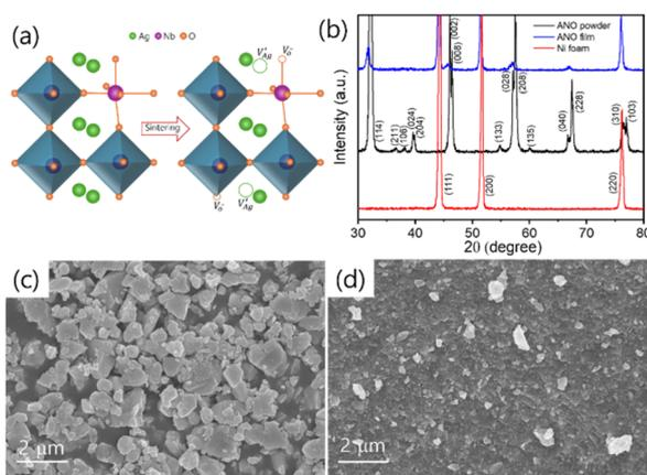
Fig. 1 (a) Schematic representation of the crystal structure of AgNbO<sub>3</sub> (ANO), highlighting the creation of oxygen vacancies. (b) XRD patterns of ANO powder, the ANO film deposited on Ni foam, and Ni foam. FESEM images of (c) ANO powder and (d) the ANO film on Ni foam.
