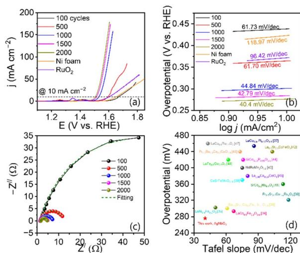
Fig. 3 OER performance of the ANO film in 1 M KOH. (a) LSV curves of ANO after various CV cycles, Ni foam and RuO<sub>2</sub>. (b) Tafel plots illustrating the kinetics of the OER, (c) EIS spectra at 0.5 V, highlighting the charge transfer resistance, (d) comparison of the OER activity of the ANO film with various perovskite oxide electrocatalysts.
