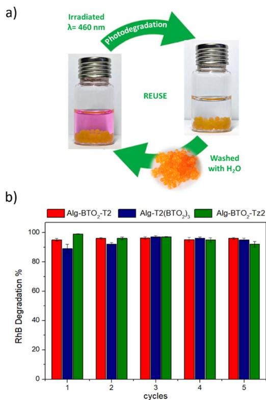
Fig. 8 (a) Sketch of the photodegradation (irradiated at  $\lambda = 460$  nm) and reuse process (aerogels washed with deionized water). (b) Recycling of Alg-BTO<sub>2</sub>-T2, Alg-T2(BTO<sub>2</sub>)<sub>3</sub> and Alg-BTO<sub>2</sub>-Tz2 aerogels on RhB showed as a case study (BPA/OFLOX, in Fig. S9, ESI†).
