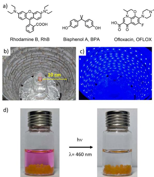
Fig. 6 (a) Chemical structure of the selected emerging contaminants (ECs), (b) photoreactor used in degradation experiments with LED off and (c) LED on. (d) Alg-BT aerogels (Alg-BTO<sub>2</sub>-T2 in the image) were suspended in contaminant spiked water (RhB case study in the image) and irradiated with blue visible light at room temperature.
