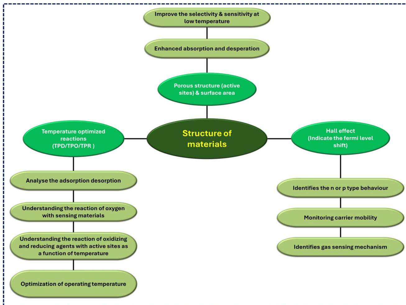
Fig. 8 A schematic diagram presents important parameters for understanding materials structures and gas sensing mechanisms, including surface area, Hall effect, and temperature-optimized reactions (TPD/TPO/TPR).
