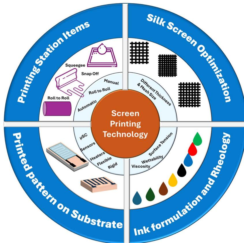
Fig. 2 Schematic diagram of screen-printing technology overview.
