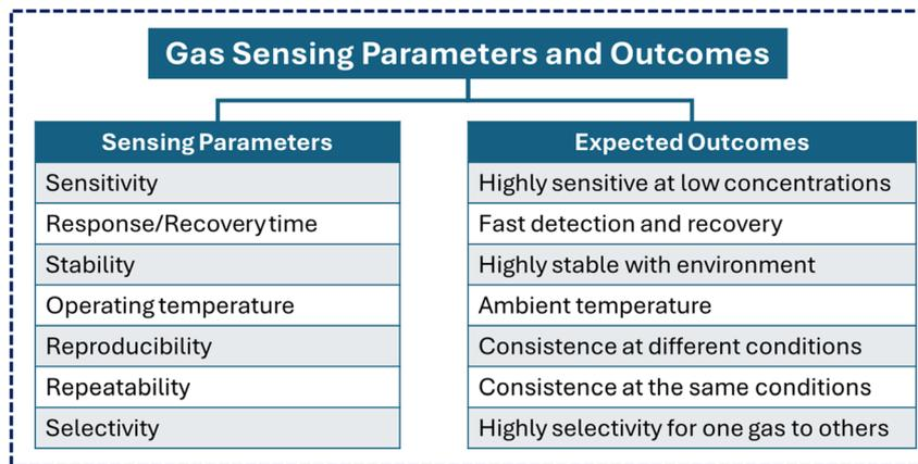
Fig. 7 Schematic diagram of gas sensing parameters and expected outcomes.
