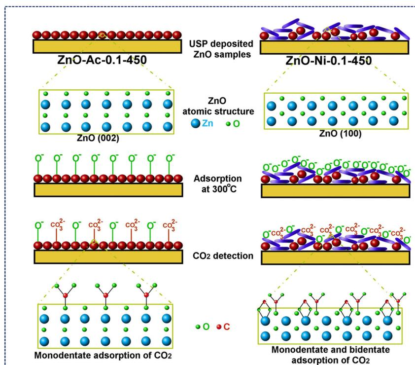
Fig. 15 CO<sub>2</sub> sensing on ZnO surfaces: zinc acetate vs. nitrate precursors. CO<sub>2</sub> gas sensing mechanism on the ZnO surfaces prepared with zinc acetate (left side) and zinc nitrate (left side) as precursors (reprinted with permission,<sup>186</sup> Copyright 2020, Springer Nature).
