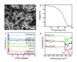
Fig. 2 (a) SEM image and (b) TGA curve of TpDB-COF. (c) PXRD patterns of TpDB-COF after treatment in various solvents, acids, and bases. (d) FT-IR spectra of TpDB-COF after treatment with 3 M HNO $_3$  and 3 M NaOH.
