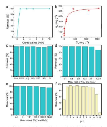
Fig. 3 (a) Adsorption kinetics of  $ReO_4^-$  by TpDB-COF. (b) Adsorption isotherm of TpDB-COF for ReO<sub>4</sub> uptake at room temperature. (c) Effect of competing anions on the removal of ReO<sub>4</sub><sup>-</sup> by TpDB-COF. Effect of excess (d)  $NO_3^-$  and (e)  $SO_4^{2-}$  on the  $ReO_4^-$  exchange. (f) Effect of pH on the removal of ReO<sub>4</sub><sup>-</sup> by TpDB-COF (initial concentration of Re:  $\sim$ 200 ppm; solid/liquid ratio of 1 mg mL<sup>-1</sup>).
