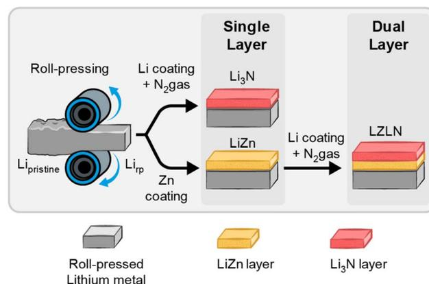
Fig. 1 *Ex situ* fabrication process for the dual protective layer starts with roll-pressing of Li metal foil to obtain  $\text{Li}_{\text{rp}}$  followed by PVD coating with either Zn or Li with subsequent  $\text{N}_2$  exposure to obtain a single protective layer. An additional  $\text{Li}_3\text{N}$  layer is deposited on top of the LiZn-intermetallic layer to form the dual protective layer.
