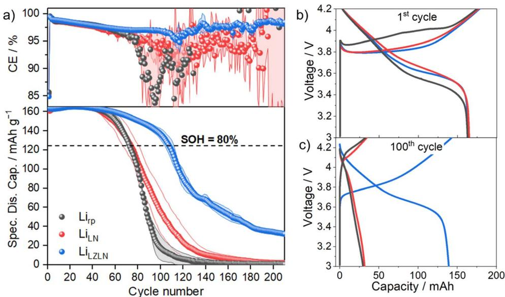
Fig. 6 (a) Electrochemical performance of NMC622||Li cells with  $\text{Li}_{\text{TP}}$  (grey),  $\text{Li}_{\text{LN}}$  (red) or  $\text{Li}_{\text{LZLN}}$  (blue) electrodes as negative electrode. (a) Capacity retention and the coulombic efficiency in a long-term cycling experiment at 0.2C. (b) The corresponding charge/discharge voltage profiles after initial cycle and (c) after 100 cycles.
