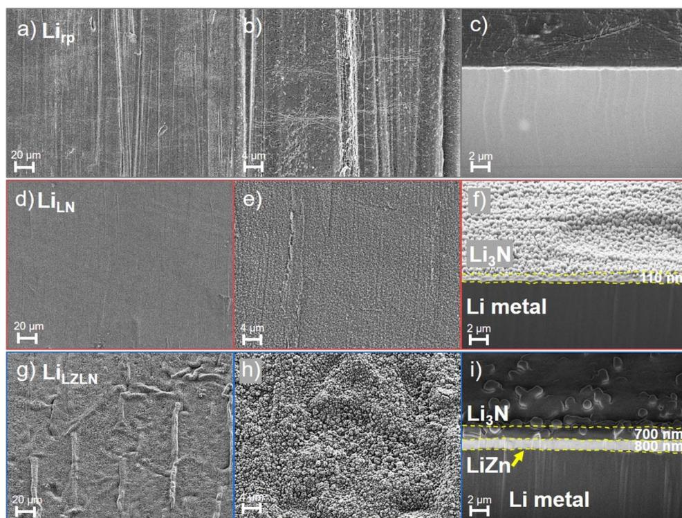
Fig. 2 Top view SEM images before cycling of (a) and (b)  $\text{Li}_{\text{rp}}$ , (d) and (e)  $\text{Li}_{\text{LN}}$  and (g) and (h)  $\text{Li}_{\text{LZLN}}$  electrodes. Cross-section images under cryogenic conditions of (c)  $\text{Li}_{\text{rp}}$ , (f)  $\text{Li}_{\text{LN}}$  at  $\text{Li}_{\text{rp}}$  and (i)  $\text{Li}_{\text{LZLN}}$ .
