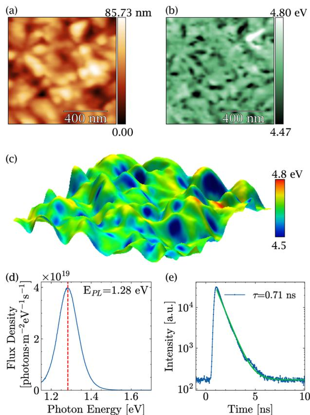
Fig. 1 Pristine MASnI<sub>3</sub>: (a) AFM topography, (b) KPFM work function measured simultaneously with the topography, (c) 3D merging of the topography and the work function with color scale, (d) PL yield and (e) TRPL.
