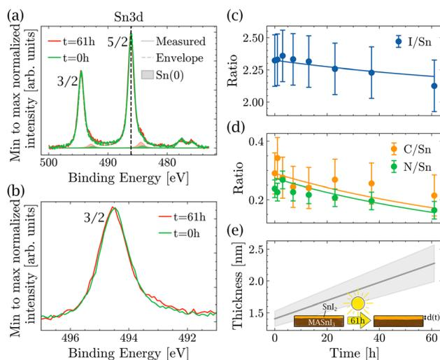
Fig. 3 Degradation of MASnI<sub>3</sub> with light over 61 h. (a) XPS measurements of the pristine sample (green) and the sample after 61 h of illumination (red) with envelope and Sn(0), and (b) zoomed-in view of the Sn 3d 3/2 peak, showing only raw data with the background subtracted. (c) Evolution of the I/Sn (c), C/Sn and N/Sn (d) ratios with the illumination time of the sample and fitting using a bi-layer model. (e) Estimation of the thickness of SnI<sub>2</sub> over time.
