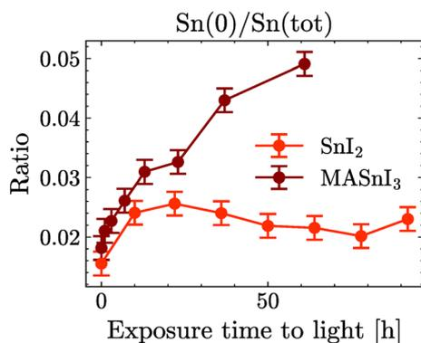
Fig. 5 Evolution of Sn(0) in MASnI<sub>3</sub> and in SnI<sub>2</sub> with light exposure.
