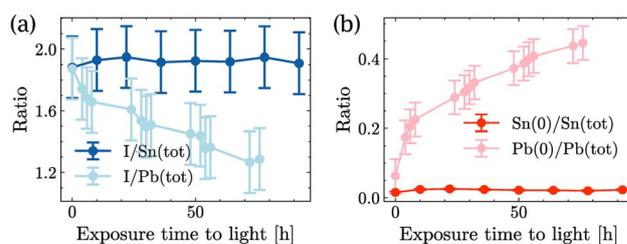
Fig. 4 Time evolution of  $\text{SnI}_2$  and  $\text{PbI}_2$  under light illumination: (a) quantity of iodide and (b) quantity of  $\text{Sn}(0)$  in  $\text{SnI}_2$  and quantity of  $\text{Pb}(0)$  in  $\text{PbI}_2$ .
