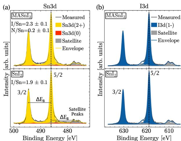
Fig. 2 Detailed XPS spectra of MASnI<sub>3</sub> (top) and SnI<sub>2</sub> (bottom) at (a) the Sn3d core-level and (b) the I3d core-level.
