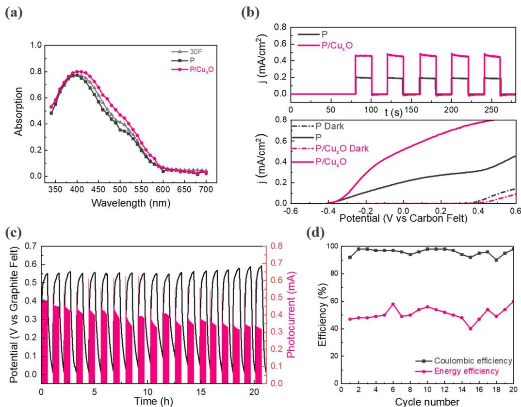
Fig. 4 (a) UV-vis absorption spectrum of nanostructures and 30F; (b) photoresponse behavior for P/Cu<sub>x</sub>O and P with 20 s light on–off; linear sweep voltammetry curve for P/Cu<sub>x</sub>O and P both under 1 sun illumination and dark; (c) representative photocharge–discharge cycling behavior with a cut-off potential set to 0–0.58 V and unbiased photocurrent using P/Cu<sub>x</sub>O photoanode; (d) coulombic and energy efficiency of photocharge/discharge curve.
