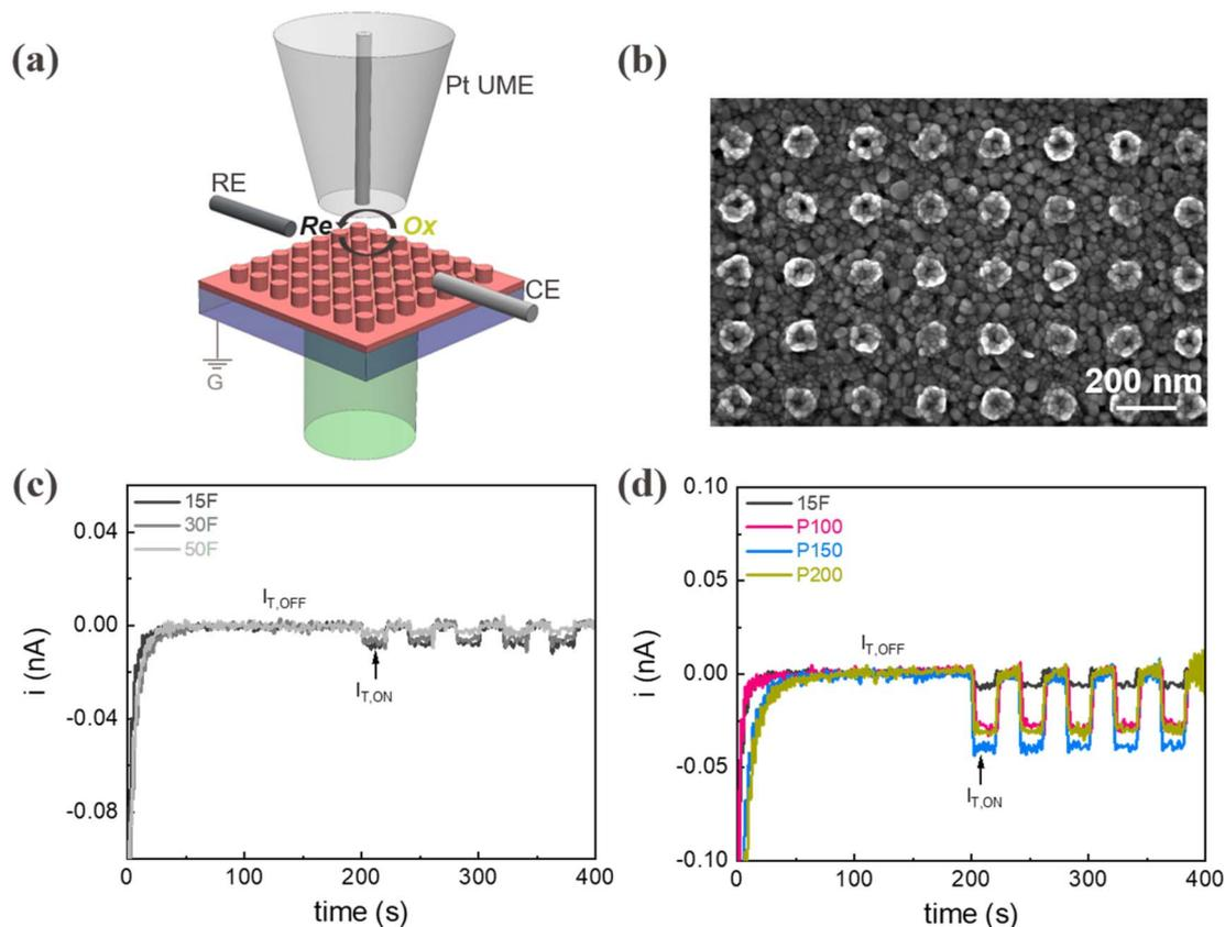
Fig. 3 (a) Schematic of light-assisted scanning electrochemical microscopy (photo-SECM) set-up, with reference electrode (RE), counter electrode (CE), reductant (Re) and oxidant (Ox); (b) SEM of P150; SECM to probe  $\alpha$ -Fe<sub>2</sub>O<sub>3</sub> (c) films (F) and (d) nanopillar arrays (P) under white light illumination (80 mW cm<sup>-2</sup>);  $I_{T,ON}$  is the current under light and  $I_{T,OFF}$  is the dark current.
