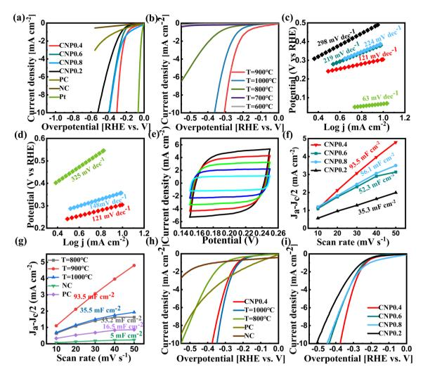
Fig. 4 (a and b) LSV curves of the various samples. (c and d) The corresponding tafel slopes. (e) CV curves of CNP0.4 in 0.5M  $H_2SO_4$  with the sweep rate changed from 10 mV s<sup>-1</sup> to 50 mV s<sup>-1</sup>. (f) ESCA of samples CNP0.2, CNP0.4, CNP0.6 and CNP0.8. (g) ESCA of sample T = 800 °C, 1000 °C, PC and NC. (h) The normalized current density of sample T = 800 °C, 900 °C, 1000 °C, PC and NC. (i) The normalized current density of CNP0.2, CNP0.4, CNP0.6 and CNP0.8.
