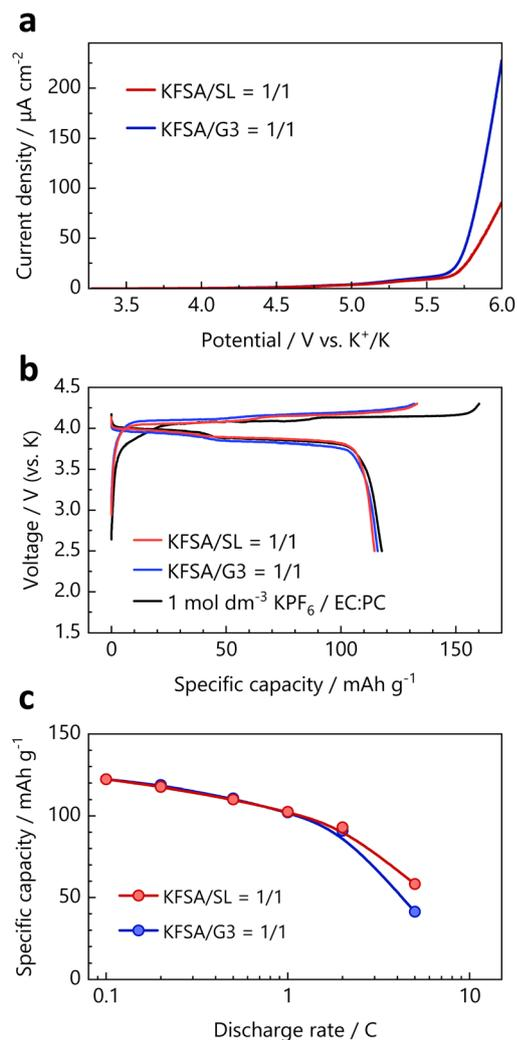
Fig. 4 (a) LSV of Pt foil in the KFSAs/SL = 1/1 and KFSAs/G3 = 1/1 electrolytes. (b) Initial charge–discharge curves of the  $\text{K}_2\text{Mn}[\text{Fe}(\text{CN})_6]$  electrodes in different electrolytes. The current density was  $15.5 \text{ mA g}^{-1}$  (corresponding to 0.1C). (c) Discharge rate dependence of the discharge capacity of the  $\text{K}_2\text{Mn}[\text{Fe}(\text{CN})_6]$  electrodes in highly concentrated electrolytes.
