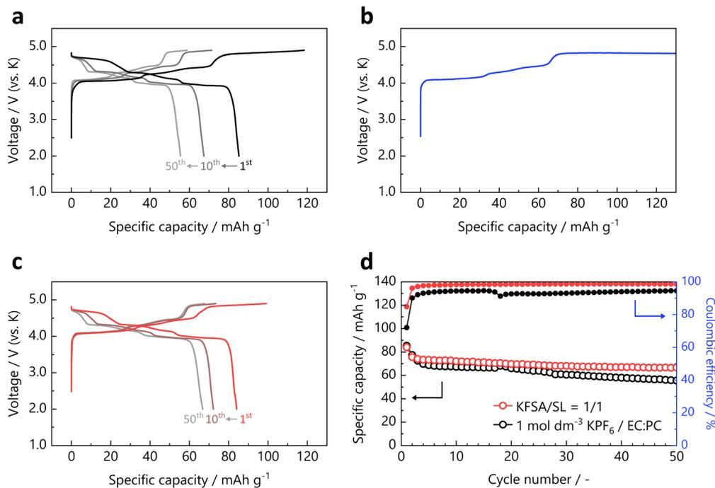
Fig. 6 Charge–discharge curves of the  $\text{KVPO}_4\text{F}$  electrodes in the (a)  $1 \text{ mol dm}^{-3} \text{ KPF}_6/\text{EC}:\text{PC}$ , (b)  $\text{KFSa}/\text{G3} = 1/1$ , and (c)  $\text{KFSa}/\text{SL} = 1/1$  electrolytes. (d) Cycling performance and coulombic efficiency of the  $\text{KVPO}_4\text{F}$  electrodes.
