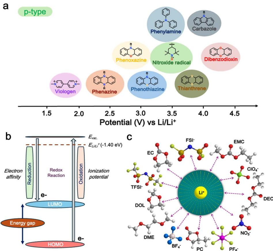
Fig. 2 (a) Different p-type organic materials along with their average redox voltages. (b) Frontier molecular orbitals (FMOs) relevant to the redox reactions of redox-active organic materials. (c) Schematic showing a solvated anion and cation within the electrolyte. Reproduced from ref. 36.
