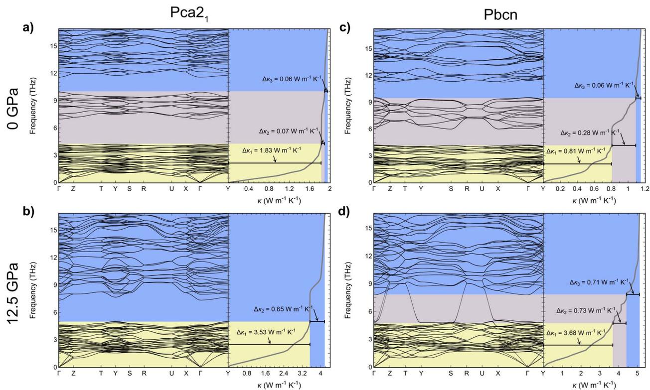
Fig. 4 Phonon dispersion curves and corresponding contributions to thermal conductivity ( $\kappa$ ) for *Pca2*<sub>1</sub> (a and b) and *Pbcn* (c and d) polymorphs at 0 and 12.5 GPa. Right-side plots show the cumulative contributions to  $\kappa$  from different frequency ranges:  $\Delta\kappa_1$ ,  $\Delta\kappa_2$  and  $\Delta\kappa_3$ .
