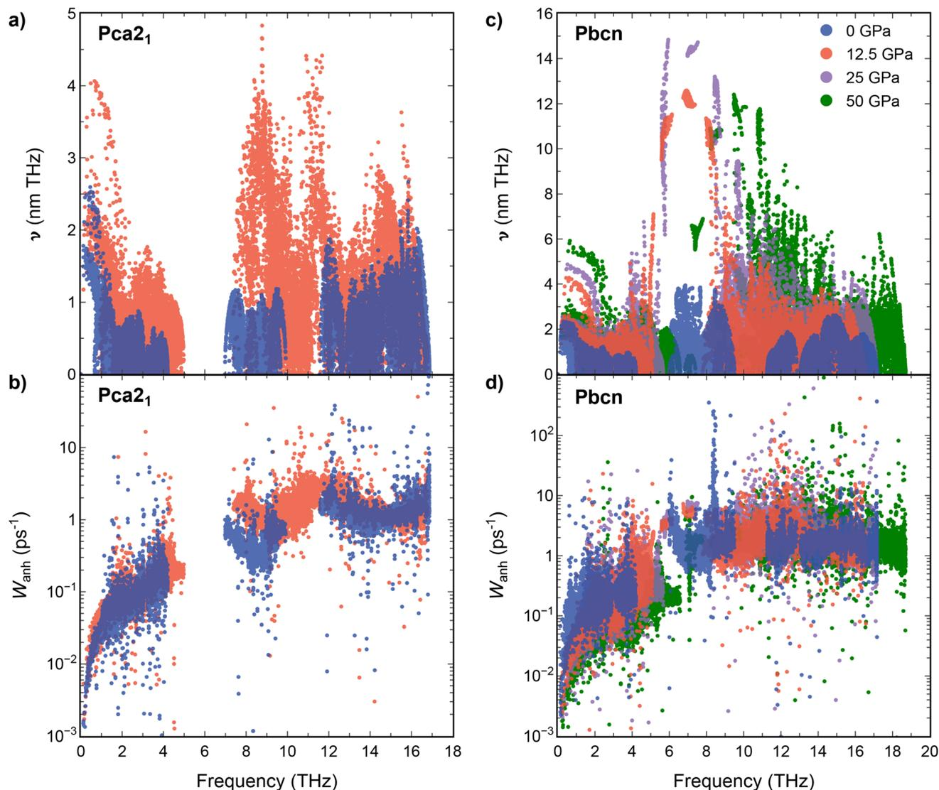
Fig. 3 Group velocities (a and c) and scattering rates (b and d) vs. frequency for *Pca2*<sub>1</sub> and *Pbcn* polymorphs at 0 (blue), 12.5 (orange), 25 (purple) and 50 (green) GPa.
