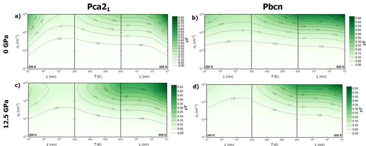
Fig. 6 Thermoelectric figure of merit ( $zT$ ) for p-type BiN as function of temperature, carrier concentration and averaged grain size. (a and b)  $zT$  for  $Pca_{21}$  and  $Pbcn$  polymorph at 0 GPa, respectively. (c and d)  $zT$  for  $Pca_{21}$  and  $Pbcn$  polymorph at 12.5 GPa, respectively.
