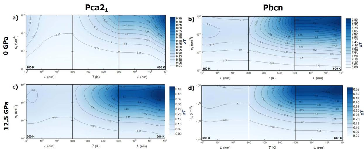
Fig. 7 Thermoelectric figure of merit ( $zT$ ) for n-type BiN as function of temperature ( $T$ ), carrier concentration ( $n$ ) and averaged grain size ( $L$ ). (a and b)  $zT$  for  $Pca_{21}$  and  $Pbcn$  polymorph at 0 GPa, respectively. (c and d)  $zT$  for  $Pca_{21}$  and  $Pbcn$  polymorph at 12.5 GPa, respectively.
