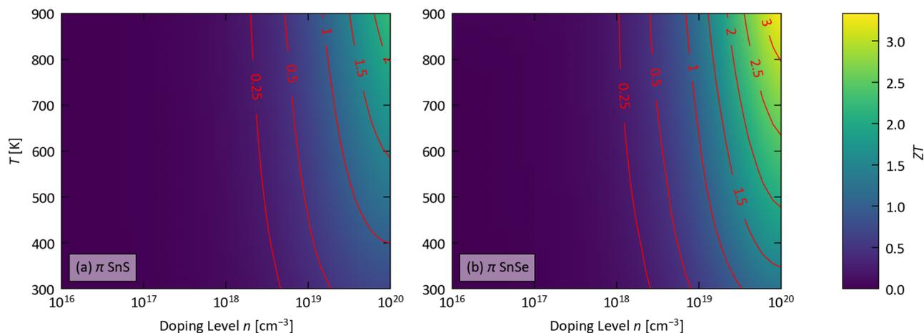
Fig. 6 Predicted thermoelectric figure of merit  $ZT$  of n-type  $\pi$  SnS (a) and SnSe (b) as a function of extrinsic electron carrier concentration  $n$  ("doping level") and temperature  $T$ . Values of  $ZT = 0.25, 0.5, 1, 1.5, 2, 2.5,$  and  $3$  are shown by contour lines.
