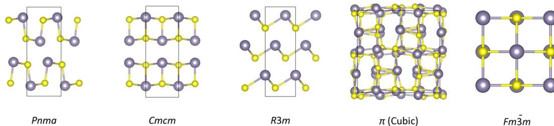
Fig. 1 Structures adopted by the group IV–VI monochalcogenides: orthorhombic *Pnma* and *Cmcm*, rhombohedral *R3m*, and cubic  $\pi$  ( $P2_13$ ) and rocksalt ( $Fm\bar{3}m$ ) phases. These images were prepared using VESTA.<sup>20</sup>
