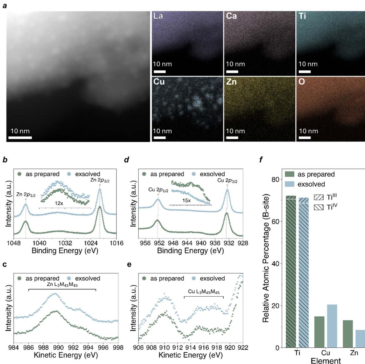
Fig. 4 Deconvoluting the Cu–ZnO relationship. (a) STEM-EDX elemental maps of La, Ca, Ti, Cu, Zn and O acquired on grains of the reduced sample. (b) Zn 2p levels. (c) Zn L<sub>3</sub>M<sub>45</sub>M<sub>45</sub>. (d) Cu 2p core levels. (e) Cu L<sub>3</sub>M<sub>45</sub>M<sub>45</sub> spectra. (f) Relative atomic percentage of the B-site components.
