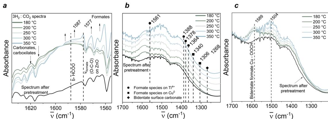
Fig. 5 Mechanistic insights into the process. *Operando* FTIR spectra for the exsolved catalyst showing the evolution of the reaction intermediates in the (a) 1630–1560  $\text{cm}^{-1}$  region, (b and c) 1700–1200  $\text{cm}^{-1}$  region highlighting the different species evolved during the *operando*  $\text{CO}_2$  hydrogenation reaction experiment (75%  $\text{H}_2$ : 25%  $\text{CO}_2$ , 7 bar, 15  $\text{mL min}^{-1}$ , NTP).
