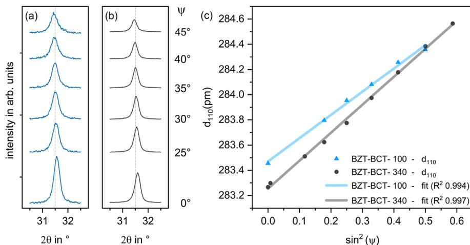
Fig. 3 Tilt-angle  $\Psi$ -dependent XRD patterns of (a) BZT–BCT-100 and (b) BZT–BCT-340 films. (c) Interplanar spacing  $d_{110}$  as a function of  $\sin^2(\Psi)$ . Different (yet both positive) slopes observed in (c) indicate different absolute values of residual biaxial strain in both films.
