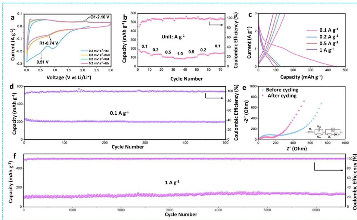
Fig. 10 Sodium storage characteristics of the VN@CF electrode: (a) CV curve at a sweep rate of  $0.2 \text{ mV s}^{-1}$ , (b) rate capability plot, (c) initial GCD profile at voltages between  $0.1$  and  $1 \text{ A g}^{-1}$ , (d) cycling behavior at a C-rate of  $0.1 \text{ A g}^{-1}$ , (e) impedance curve for the device before and after testing, and (f) cycling behavior at a C-rate of  $1 \text{ A g}^{-1}$ , reproduced with permission from ref. 104, Copyright 2023, Elsevier.
