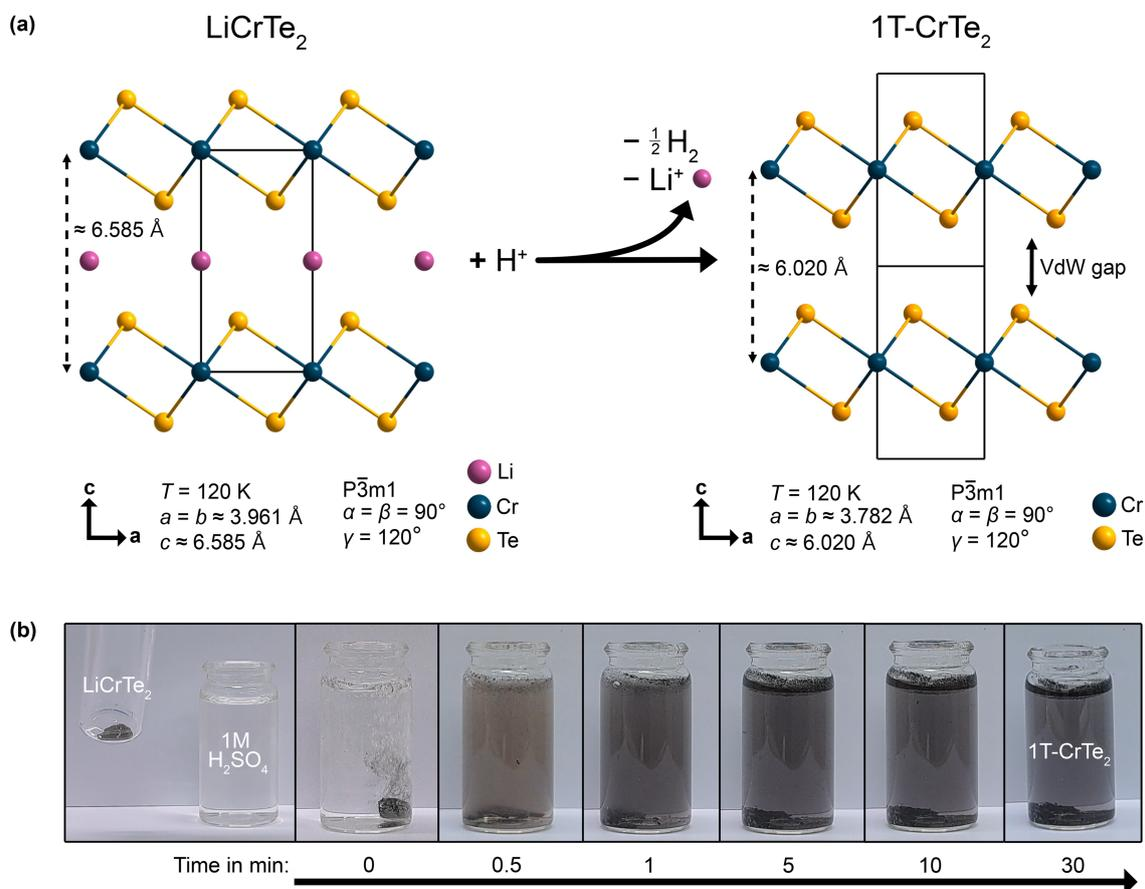
Fig. 1 Acid-assisted synthesis of 1T-CrTe<sub>2</sub>: (a) Scheme of the deintercalation reaction of LiCrTe<sub>2</sub> with an acid and the respective cell parameters of LiCrTe<sub>2</sub> (ref. 56) based on synchrotron data and 1T-CrTe<sub>2</sub> based on our SXRD data. (b) Images of the deintercalation process of LiCrTe<sub>2</sub> crystals in diluted 1 M H<sub>2</sub>SO<sub>4</sub> with the respective time stamps.
