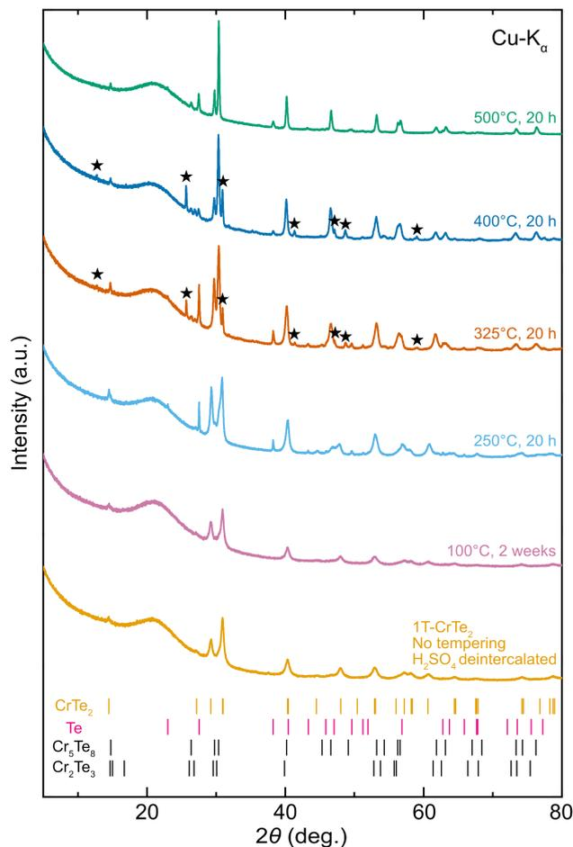
Fig. 8 PXRD patterns showing the thermal stability of 1T-CrTe<sub>2</sub> after tempering at 100 °C for two weeks, and at 250 °C, 325 °C, 400 °C, and 500 °C for 20 hours. Stars indicate an unidentified phase, potentially resembling CrTe<sub>3</sub>, and Bragg positions of identified phases are shown below the patterns.
