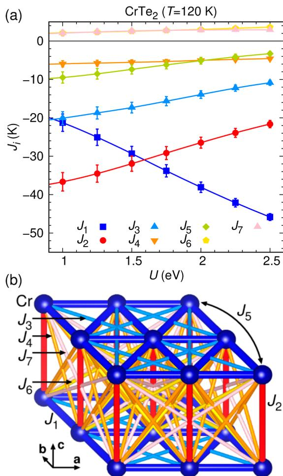
Fig. 7 (a) Exchange interactions of 1T-CrTe<sub>2</sub> determined by DFT energy mapping using a DFT + U exchange correlation functional, as function of the on-site interaction strength  $U$ . (b) Seven relevant exchange paths for CrTe<sub>2</sub>.
