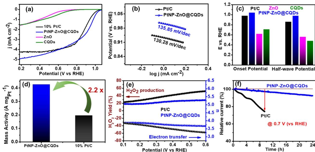
Fig. 5 (a) CLSV curve of PtNP-ZnO@CQD, ZnO, CQD, commercial Pt/C catalysts. (b) Tafel slope of the catalysts. (c) Bar diagram to compare different catalysts' onset and half-wave potentials. (d) Bar diagram to compare the mass activity of different catalysts. (e) Number of electrons transferred and  $\text{H}_2\text{O}_2$  yield of PtNP-ZnO@CQD and Pt-carbon catalysts. (f) Chronoamperometric plot of PtNP-ZnO@CQD and Pt/C catalysts during the ORR.
