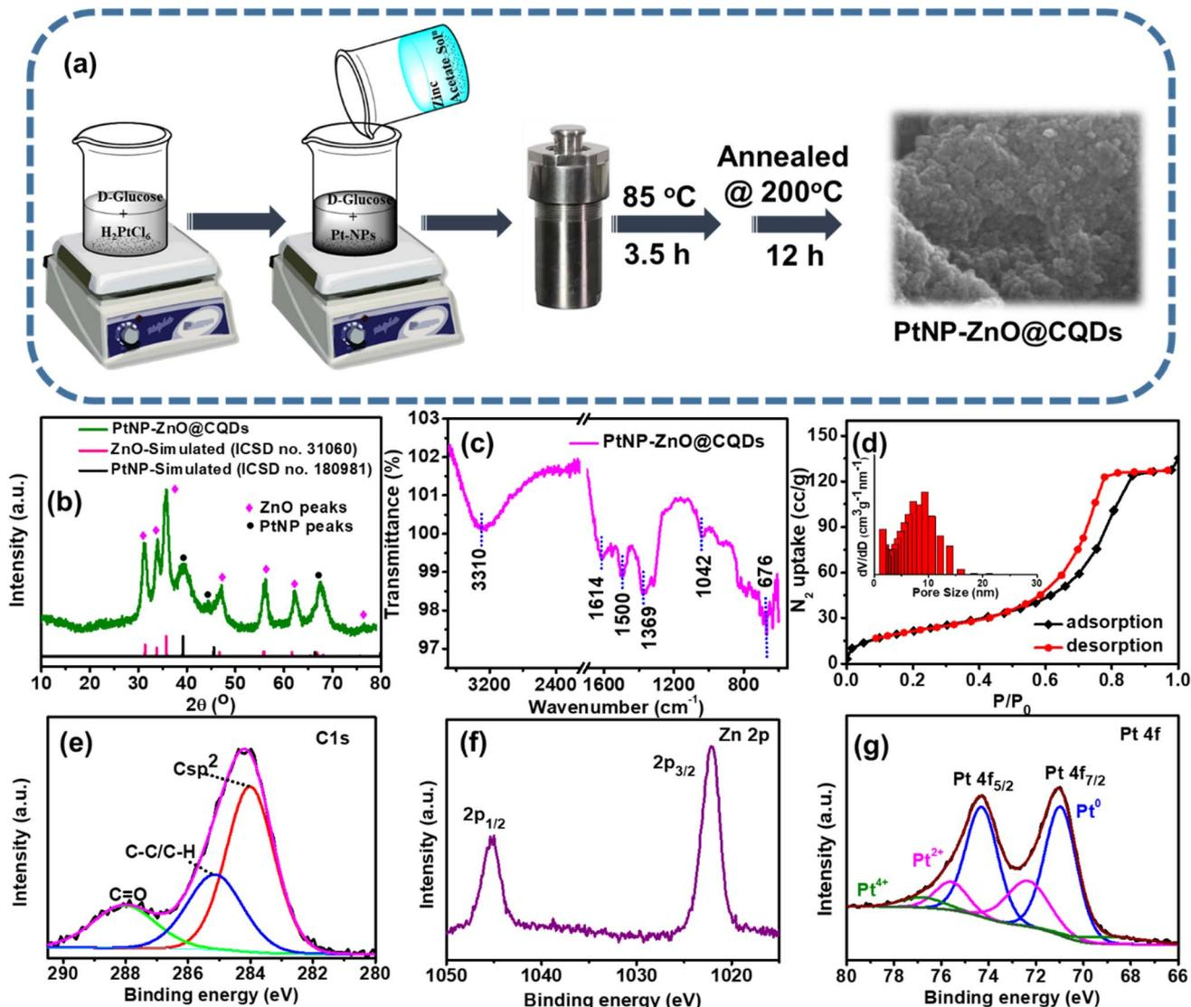
Fig. 1 (a) Schematic diagram of the synthesis of PtNP-ZnO@CQDs. (b) X-ray diffraction pattern of PtNP-ZnO@CQDs compared with simulated ZnO and PtNP patterns. (c) FT-IR of PtNP-ZnO@CQDs. (d)  $N_2$ -isotherm of PtNP-ZnO@CQDs. The pore size distribution plot is given in the inset. Core level XPS spectra of (e) C 1s, (f) Zn 2p, and (g) Pt 4f.
