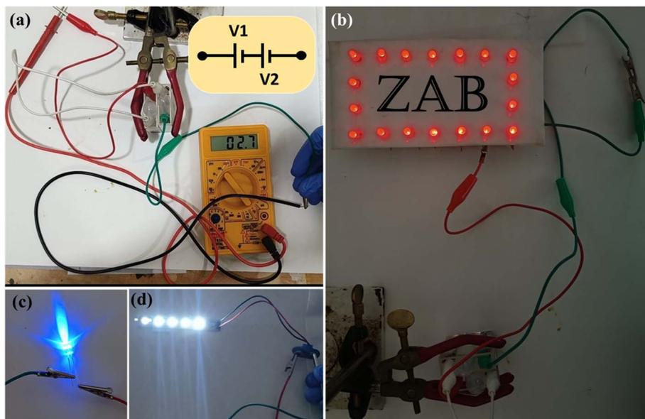
Fig. 7 (a) The assembled ZABs are made up of PtNP-ZnO@CQD catalysts in a series combination. The assembled ZAB lights of (b) a 1.8 V red LED light panel, (c) a 3.4 V blue LED light and (d) a 6 V white LED light.
