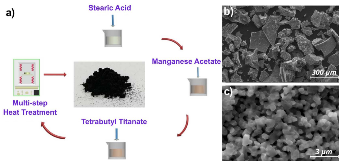
Fig. 1 (a) Schematic synthesis route for the synthesis of \text{MnTiO}_3 powders, (b) low magnification, and (c) high magnification FESEM images for the \text{MnTiO}_3 powders.
