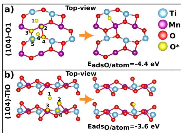
Fig. 4 Top views of (a) O1 and (b) TiO terminations of  $\text{MnTiO}_3$  (104). In the left, the tested initial adsorption sites for oxygen atoms are shown, while in the right, the geometry after structural optimization is presented. The adsorption energies are given per adsorbed oxygen atom.
