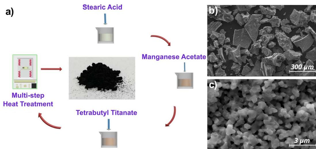
Fig. 1 (a) Schematic synthesis route for the synthesis of MnTiO<sub>3</sub> powders, (b) low magnification, and (c) high magnification FESEM images for the MnTiO<sub>3</sub> powders.
