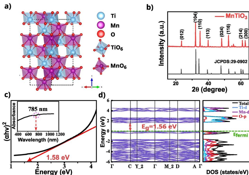
Fig. 2 (a) The crystal structure of  $\text{MnTiO}_3$  with a trigonal unit cell. (b) The XRD patterns of  $\text{MnTiO}_3$ , (c)  $(\alpha h\nu)^2 - h\nu$  curves of the  $\text{MnTiO}_3$  powders, and the corresponding absorption spectra in the inset obtained from the UV-visible measurements, (d) the calculated band structure, band gap ( $E_g$ ), and the orbital-projected density of states (PDOS) from DFT.
