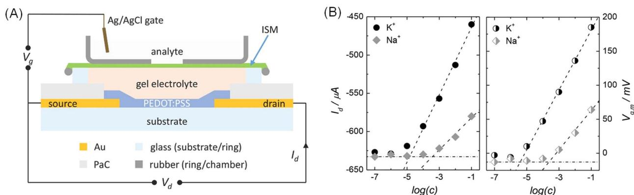
Fig. 7 (A) Schematic of  $K^+$ -selective OECTs. (B) Calibration curves of different ionic solutions obtained using  $K^+$ -selective OECTs. Reproduced with permission.<sup>39</sup> Copyright 2014, Wiley-VCH.
