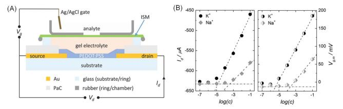
Fig. 7 (A) Schematic of  $K^+$ -selective OECTs. (B) Calibration curves of different ionic solutions obtained using  $K^+$ - selective OECTs. Reproduced with permission.<sup>39</sup> Copyright 2014, Wiley-VCH.
