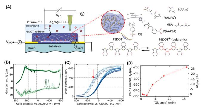
Fig. 9 (A) Schematic and mechanism of DN hydrogel-based OECTs for glucose sensing. The concurrent gate leakage (B) and transfer curves (C) during glucose sensing (darker shades and dot-dashed curves correspond to high and low glucose concentration, responsively). (D) Extracted from the midpoint potential of the ROI as indicated by the red arrow in (C). Reproduced with permission.<sup>42</sup> Copyright 2022, American Chemical Society.
