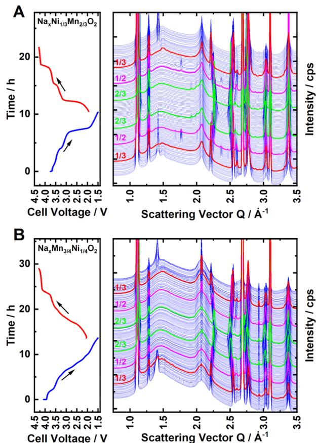
Fig. 4 Synchrotron *operando* XRD for (A)  $\text{Na}_{2/3}\text{Ni}_{1/3}\text{Mn}_{2/3}\text{O}_2$  and (B)  $\text{Na}_{0.60}\text{Mn}_{3/4}\text{Ni}_{1/4}\text{O}_2$ . Both measurements were started in a charged state. The diffraction patterns corresponding to sodium stoichiometries of  $x = 1/3$ ,  $1/2$  and  $2/3$  are highlighted in red, magenta and green colour, respectively.
