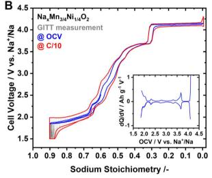
Fig. 3 GITT measurements for (A)  $Na_{2/3}Ni_{1/3}Mn_{2/3}O_2$  and (B) Na<sub>0.60</sub>Mn<sub>3/4</sub>Ni<sub>1/4</sub>O<sub>2</sub> as CAM. The OCV for various stoichiometries is highlighted as a blue hull curve, and the on-load hull curve is highlighted in red colour. For both materials, dQ/dV analysis of the OCV curve is included in the inset.
