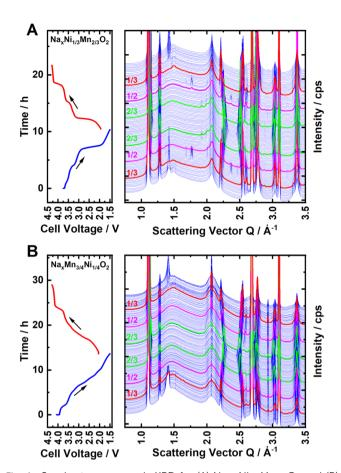
Fig. 4 Synchrotron operando XRD for (A)  $Na_{2/3}Ni_{1/3}Mn_{2/3}O_2$  and (B)  $Na_{0.60}Mn_{3/4}Ni_{1/4}O_2$ . Both measurements were started in a charged state. The diffraction patterns corresponding to sodium stoichiometries of x=1/3, 1/2 and 2/3 are highlighted in red, magenta and green colour, respectively.
