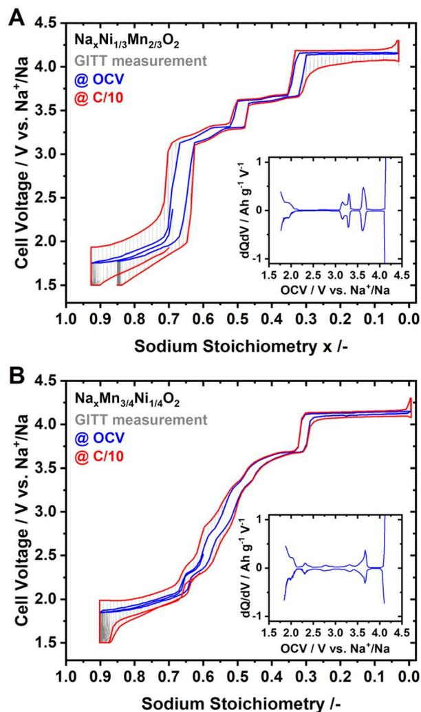
**Fig. 3** GITT measurements for (A)  $\text{Na}_{2/3}\text{Ni}_{1/3}\text{Mn}_{2/3}\text{O}_2$  and (B)  $\text{Na}_{0.60}\text{Mn}_{3/4}\text{Ni}_{1/4}\text{O}_2$  as CAM. The OCV for various stoichiometries is highlighted as a blue hull curve, and the on-load hull curve is highlighted in red colour. For both materials,  $dQ/dV$  analysis of the OCV curve is included in the inset.
