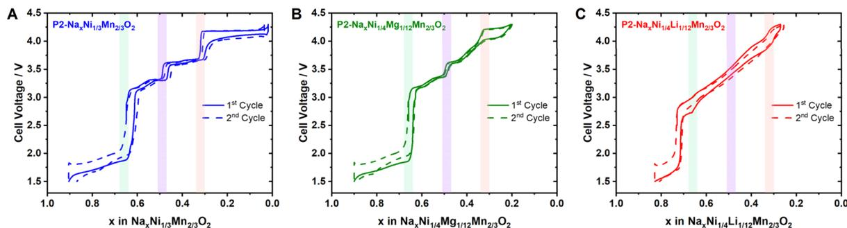
Fig. 11 Potential profile for the first two full galvanostatic cycles of (A)  $\text{P2-Na}_x\text{Ni}_{1/3}\text{Mn}_{2/3}\text{O}_2$ , (B)  $\text{P2-Na}_x\text{Ni}_{1/4}\text{Mg}_{1/12}\text{Mn}_{2/3}\text{O}_2$  and (C)  $\text{Na}_{3/4}\text{Ni}_{1/4}\text{Li}_{1/12}\text{Mn}_{2/3}\text{O}_2$  as cathode materials in a sodium half-cell.
