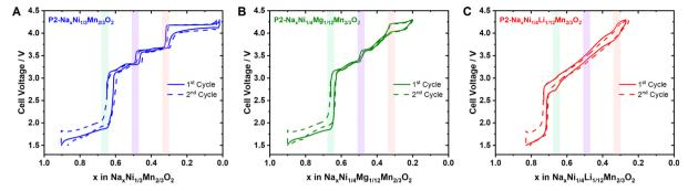
Fig. 11 Potential profile for the first two full galvanostatic cycles of (A) P2-Na<sub>2/3</sub>Ni<sub>1/3</sub>Mn<sub>2/3</sub>O<sub>2</sub>, (B) P2-Na<sub>2/3</sub>Ni<sub>1/4</sub>Mg<sub>1/12</sub>Mn<sub>2/3</sub>O<sub>2</sub> and (C) Na<sub>3/4</sub>Ni<sub>1/4</sub>  $_{4}\text{Li}_{1/12}\text{Mn}_{2/3}\text{O}_{2}$  as cathode materials in a sodium half-cell.
