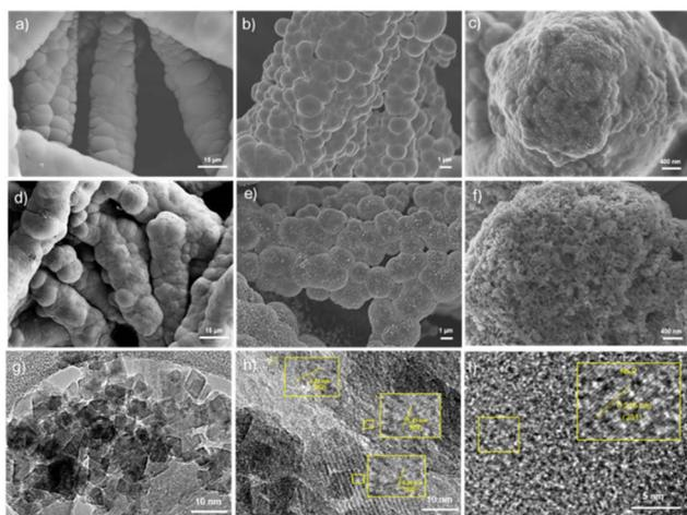
Fig. 2 High-resolution scanning electron microscopy images of the (a–c) CFP/Ni<sub>3</sub>P, and (d–f) CFP/Ni<sub>3</sub>P/ $\delta$ -FeOOH samples. (g–i) HRTEM images of the  $\delta$ -FeOOH and Ni<sub>3</sub>P samples.
