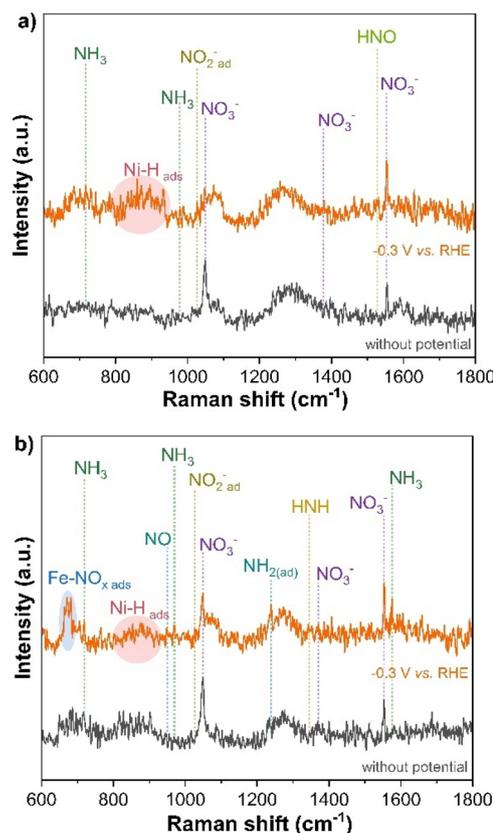
Fig. 6 Operando Raman spectra without applied potential and at  $-0.3$  V vs. RHE for (a) CFP/Ni<sub>3</sub>P and (b) CFP/Ni<sub>3</sub>P/δ-FeOOH.
