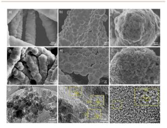
Fig. 2 High-resolution scanning electron microscopy images of the (a-c) CFP/Ni<sub>3</sub>P, and (d-f) CFP/Ni<sub>3</sub>P/δ-FeOOH samples. (g-i) HRTEM images of the δ-FeOOH and Ni<sub>3</sub>P samples.
