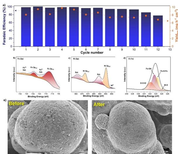
Fig. 5 (a) Consecutive recycling test of the CFP/Ni<sub>3</sub>P/δ-FeOOH electrode at  $-0.3$  V vs. RHE. XPS spectra of the CFP/Ni<sub>3</sub>P/δ-FeOOH sample after 10 consecutive recycling cycles: (b) Fe 2p, (c) Ni 2p, and (d) O 1s. (e) High-resolution scanning electron microscopy images of the CFP/Ni<sub>3</sub>P/δ-FeOOH sample freshly prepared and after the recycling cycles.
