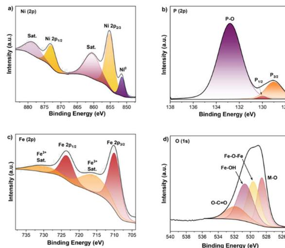
Fig. 3 XPS analysis of the CFP/Ni<sub>3</sub>P/ $\delta$ -FeOOH sample: (a) Ni 2p, (b) P 2p, (c) Fe 2p, and (d) O 1s.
