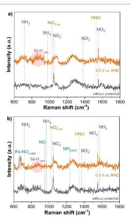
Fig. 6 Operando Raman spectra without applied potential and at -0.3 V vs. RHE for (a) CFP/Ni<sub>3</sub>P and (b) CFP/Ni<sub>3</sub>P/ $\delta$ -FeOOH.
