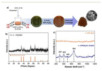
Fig. 1 (a) Schematic diagram of the  $\delta$ -FeOOH sample synthesis. (b) XRD pattern of the  $\delta$ -FeOOH sample. (c) Raman spectra of the CFP/Ni<sub>3</sub>P and CFP/Ni<sub>3</sub>P/ $\delta$ -FeOOH electrodes.
