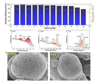
Fig. 5 (a) Consecutive recycling test of the CFP/Ni<sub>3</sub>P/δ-FeOOH electrode at -0.3 V vs. RHE. XPS spectra of the CFP/Ni<sub>3</sub>P/ $\delta$ -FeOOH sample after 10 consecutive recycling cycles: (b) Fe 2p, (c) Ni 2p, and (d) O 1s. (e) High-resolution scanning electron microscopy images of the CFP/Ni<sub>3</sub>P/δ-FeOOH sample freshly prepared and after the recycling cycles.
