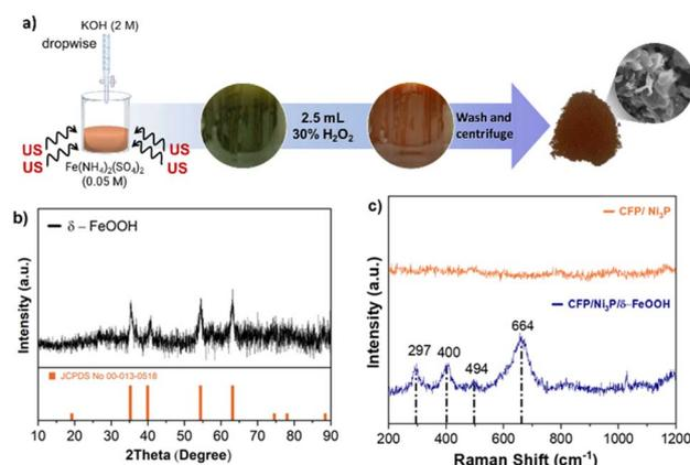
Fig. 1 (a) Schematic diagram of the δ-FeOOH sample synthesis. (b) XRD pattern of the δ-FeOOH sample. (c) Raman spectra of the CFP/Ni<sub>3</sub>P and CFP/Ni<sub>3</sub>P/δ-FeOOH electrodes.
