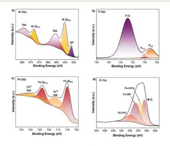
Fig. 3 XPS analysis of the CFP/Ni<sub>3</sub>P/δ-FeOOH sample: (a) Ni 2p, (b) P 2p, (c) Fe 2p, and (d) O 1s.
