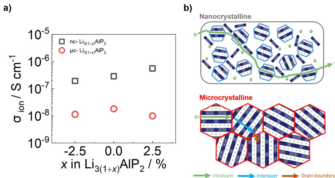
Fig. 10 (a) Ionic conductivities and (b) cartoon schematics for ion transport processes in  $\text{nc-Li}_3\text{AlP}_2$  and  $\mu\text{c-Li}_3\text{AlP}_2$  materials.
