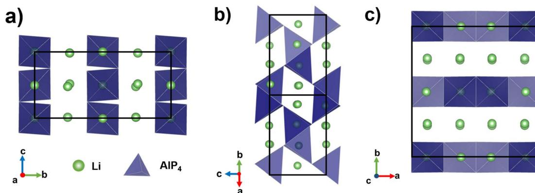
Fig. 1 Crystal structure of orthorhombic  $\text{Li}_3\text{AlP}_2$ ,<sup>16</sup> the unit cell is shown in solid black lines.  $\text{AlP}_4$  tetrahedra are shown in blue and Li atoms in green.  $\text{Li}^+$  layers in the  $a$  and  $c$  axes are notable in (a) and (c). Intralayer  $\text{Li}^+$  channels are highlighted in (b).
