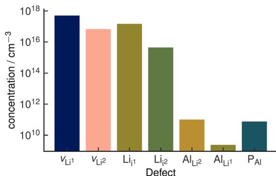
Fig. 5 Defect concentrations in orthorhombic  $\text{Li}_3\text{AlP}_2$  calculated under thermodynamic equilibrium. The two unique Li sites are discretised with the notation site  $\text{Li}^1$  and site  $\text{Li}^2$ . Site  $\text{Li}^1$  refers to the lithium site in the Li layer. Site  $\text{Li}^2$  refers to the lithium site in the mixed Li/Al layer. The positions of the two interstitial sites are shown in the ESI, Fig. S1.†
