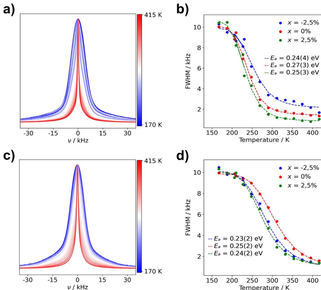
Fig. 8 Normalized static  ${}^7\text{Li}$  NMR spectra and FWHM of  $\text{Li}_{3(1+x)}\text{AlP}_2$  for (a)  $\mu\text{c-Li}_{2.925}\text{AlP}_2$   ${}^7\text{Li}$  NMR spectra (b)  $\mu\text{c-Li}_{3(1+x)}\text{AlP}_2$  FWHM fit with eqn (1) and (c)  $\text{nc-Li}_{2.925}\text{AlP}_2$  (d)  $\text{nc-Li}_{3(1+x)}\text{AlP}_2$  FWHM fit with eqn (1). The used color gradient ranges from blue (low temperatures) to red (high temperatures) to indicate the change of lineshapes with temperature.
