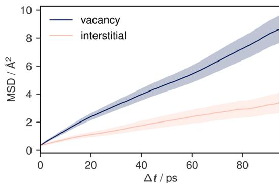
Fig. 2 Mean squared displacement plots for two 95 ps simulations of  $\text{Li}_3\text{AlP}_2$  simulated at 900 K. One simulation cell contains a vacancy and the other, an interstitial. The shaded areas show a 95% confidence interval in the mean-squared displacement.
