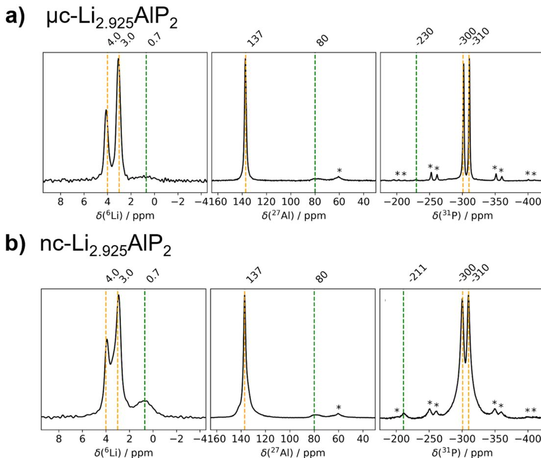
Fig. 7  ${}^6\text{Li}$ ,  ${}^{27}\text{Al}$  and  ${}^{31}\text{P}$  MAS NMR spectra of  $\text{Li}_{3(1+x)}\text{AlP}_2$ . (a)  $\mu\text{c-Li}_{2.925}\text{AlP}_2$  and (b)  $\text{nc-Li}_{2.925}\text{AlP}_2$  recorded with a MAS frequency of 10.0 kHz (11.75 T).
