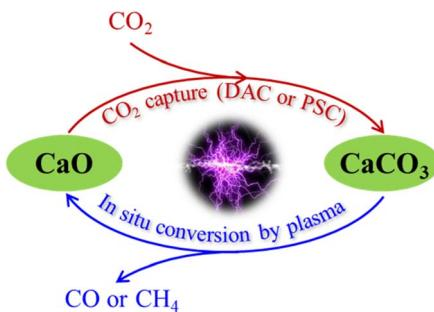
Nonthermal plasma assisted desorption and conversion of captured  $\text{CO}_2$  from atmospheric air
