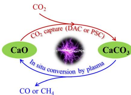
Nonthermal plasma assisted desorption and conversion of captured  $\text{CO}_2$  from atmospheric air
