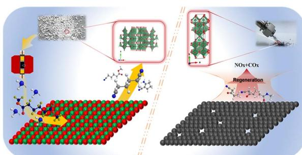
Deactivation mechanisms of  $\text{Nb}_2\text{O}_5$  catalyst for esterification of dimethyl adipate: crystal transformation and acid site coking
