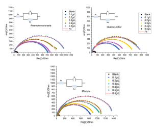
Fig. 5 Nyquist plots of the MS in the presence and the absence of various amounts of AC, QR and mixture in 1 M HCl at 293 K.
