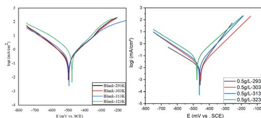
Fig. 9 The PDP plots of MS in 1 M HCl + 0.5 g L<sup>-1</sup> of the mixture at different temperatures.
