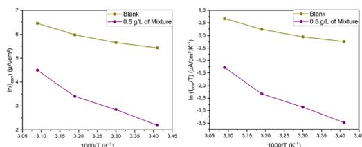
Fig. 10 (Left) Arrhenius plots and (Right) transition state plots of MS in 1 M HCl in the absence and presence of 0.5 g L<sup>-1</sup> of inhibitor.
