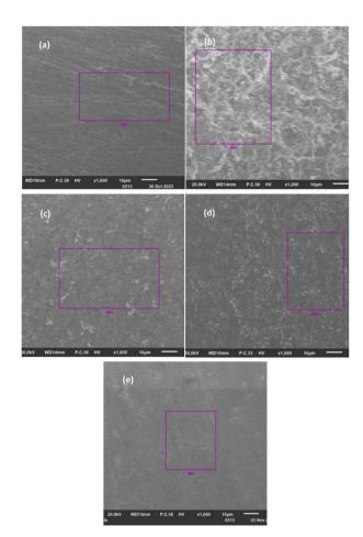
Fig. 8 SEM images of (a) polished steel (b) steel immersed in uninhibited 1 M HCl (c) steel immersed in 1 M HCl + Anemone coronaria (d) steel immersed in 1 M HCl + Quercus robur (e) steel immersed in 1 M HCl + mixture.
