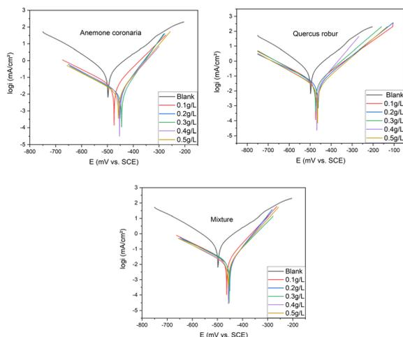
Fig. 4 PDP curves of the MS in HCl medium with varying concentrations of AC, QR and mixture.
