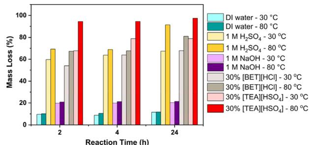
Fig. 2 Mass loss after treatment of BM with DI water, 1 M H<sub>2</sub>SO<sub>4</sub>, 1 M NaOH, 30% [Bet][HCl] and 30% [TEA][H<sub>2</sub>SO<sub>4</sub>] at 2 h, 4 h and 24 h.
