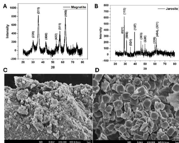
Fig. 1 XRD patterns of the greenly synthesized (A) magnetite and (B) jarosite. Scanning Electron Microscopy (SEM) images of the greenly synthesized (C) magnetite and (D) jarosite. Scale bar: 1  $\mu\text{m}$ .
