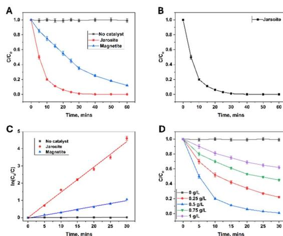
Fig. 4 (A and B) Photodegradation plots of RhB, (C) reaction kinetic plots, and (D) effect of jarosite concentration on RhB photodegradation.
