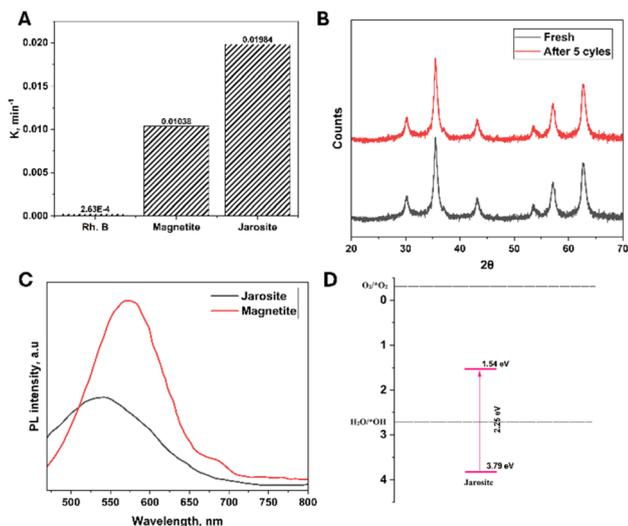
Fig. 5 (A) Pseudo-1st-order rate constants of the photocatalysts. (B) XRD patterns of jarosite before and after 5 cycles of the photocatalytic reaction. (C) Photoluminescence spectra of jarosite (black line) and magnetite (red line). (D) Energy band positions of jarosite.
