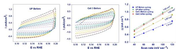
Fig. 4 CVs recorded from 40 to 120 mV s<sup>-1</sup> in 1 M KOH at UP (NMC-622) and NMC 622 recovered from Cell 3. Also shown are plots determining the ECSA for UP and Cell 3 before the OER and after being subjected to 2000 cycles in the OER region (1 to 1.9 V).
