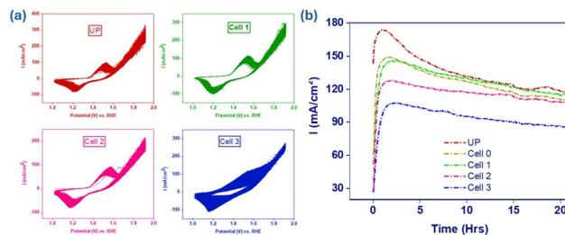
Fig. 2 (a) Cyclic voltammograms recorded at  $100 \text{ mV s}^{-1}$  for 2000 cycles and (b) chronoamperometric experiments conducted at 1.7 V for 21 h for UP, Cell 0, Cell 1, Cell 2 and Cell 3 electrodes in 1 M KOH.
