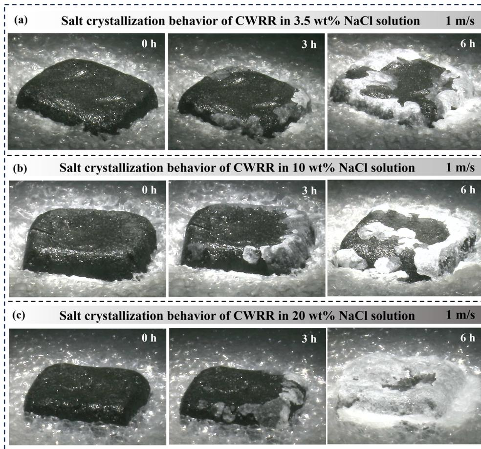
Fig. 6 Distribution of salt accumulation. Digital images of CWRR in (a) 3.5, (b) 10, and (c) 20 wt% NaCl at a wind speed of  $1 \text{ m s}^{-1}$ . The CWRR samples in the figures all consisted of cubic blocks with a length and width of  $2 \text{ cm} \times 2 \text{ cm}$ .
