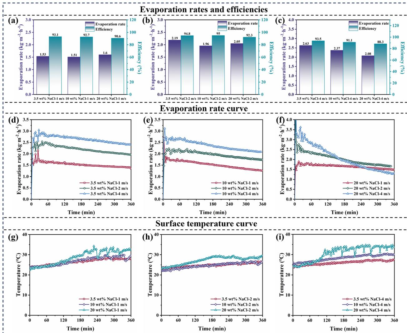
Fig. 5 Evaporation performances of CWRR under different convective airflows. Evaporation rates and efficiencies of CWRR in 3.5, 10, and 20 wt% NaCl at (a) 1, (b) 2, and (c) 4 m s<sup>-1</sup> wind speeds over 6 hours. Evaporation rate curves of CWRR in 3.5, 10, and 20 wt% NaCl at (d) 1, (e) 2, and (f) 4 m s<sup>-1</sup> wind speeds over 6 hours. Temperature change curves of CWRR in 3.5, 10, and 20 wt% NaCl at (g) 1, (h) 2, and (i) 4 m s<sup>-1</sup> wind speeds over 6 hours.
