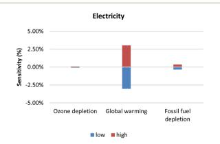
Fig. 5 Sensitivity analysis results indicate that electricity usage in the whole process is the primary contributor to high environmental impacts.
