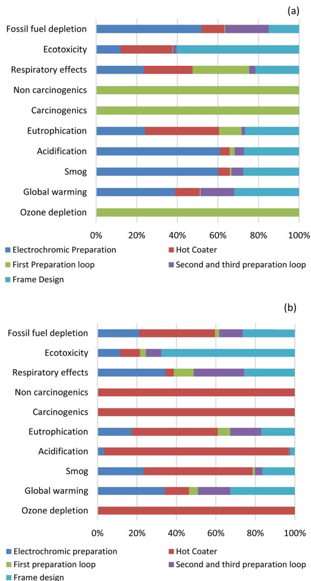
Fig. 6 Contribution of process energy and material flows in all stages of 1 m<sup>2</sup> EC glass production using (a) PyTorch's ANN model and (b) PyTorch's three-level ANFIS model.
