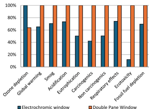
Fig. 4 A comparison between EC windows and DP windows based on the environmental impacts resulting from the production of 1 m<sup>2</sup> of them using TRACI.
