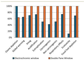
Fig. 4 A comparison between EC windows and DP windows based on the environmental impacts resulting from the production of 1  $\rm m^2$  of them using TRACI.
