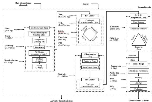
Fig. 1 Simplified system boundary to produce a 1 m<sup>2</sup> EC window (no wastes and co-products considered).
