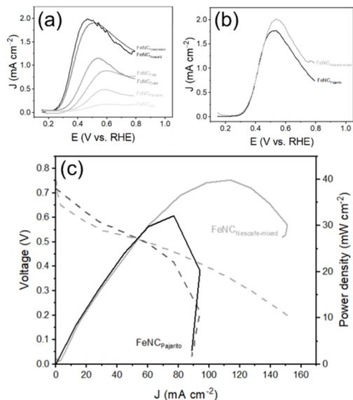
Fig. 2 (a) Linear sweep voltammograms of hydrazine oxidation on six coffee-waste-derived FeNC catalysts (20 mM  $\text{N}_2\text{H}_4$ , 1 M KOH, 10  $\text{mV s}^{-1}$ ). (b) LSVs on  $\text{FeNC}_{\text{Nescafe-mixed}}$  and commercial  $\text{FeNC}_{\text{Pajarito}}$ . (c) Direct hydrazine fuel cell polarization curves with  $\text{FeNC}_{\text{Nescafe-mixed}}$  or  $\text{FeNC}_{\text{Pajarito}}$  anodes and a PGM-free cathode, at 80 °C (see the SI for details).
