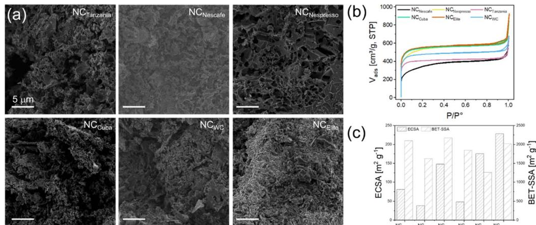
Fig. 1 (a) Characteristic scanning electron micrographs of the coffee-derived carbons. (b) N<sub>2</sub> sorption isotherms at 77 K. (c) Specific surface areas (SSAs-BET) and electrochemical surface areas (ECSAs) of the carbons.
