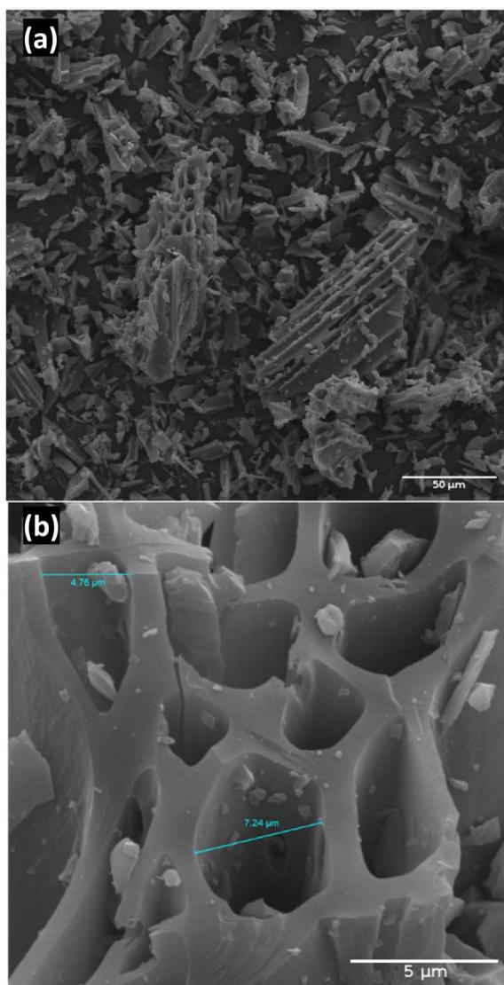
Fig. 6 Morphology of (a) activated biochar produced at 650 °C (ABC650) displayed at a magnification of 1 k and a scale of 50  $\mu\text{m}$ , showing a fragmented structure with irregular and rough surfaces; (b) detailed view of the porous structure of ABC650 sample displayed at a magnification of 10 k and a scale of 5  $\mu\text{m}$ .
