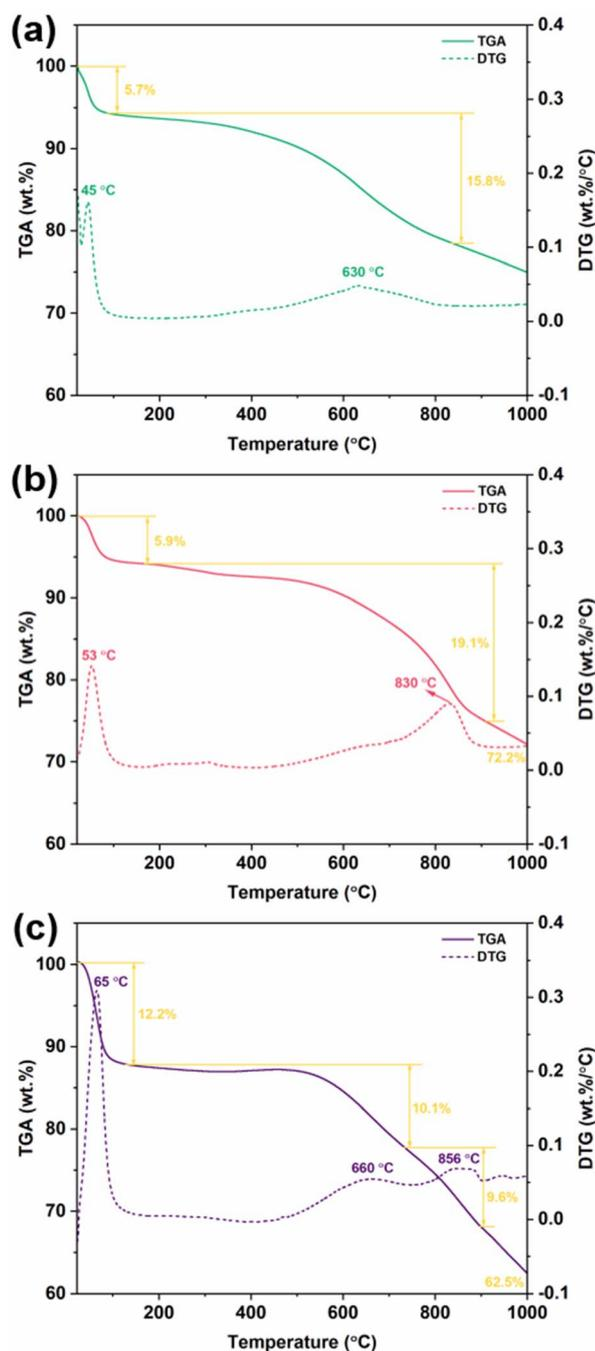
Fig. 5 Thermogravimetry analysis (TGA, solid lines) and derivative thermogravimetry (DTG, dashed lines) curves of (a) BC, (b) ABC550, and (c) ABC650 biochar materials.
