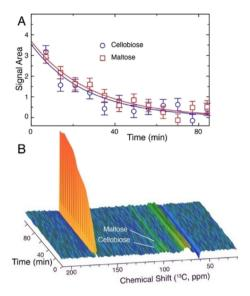
Fig. 4 Competition experiment for the one-pot conversion of maltose and cellobiose. Integrals of the substrates (A) are shown alongside the time series of DEPT135 <sup>13</sup>C NMR spectra (B). Reaction conditions: 0.025 M cellobiose and 0.025 M maltose, 0.6 M LiOH and 24 equiv. hydrogen peroxide in a 3 mm NMR tube (200 μL H<sub>2</sub>O/D<sub>2</sub>O (90%/10%)) at 308 K without agitation.
