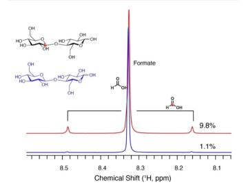
Fig. 7 Reaction conditions: 0.05 M cellobiose or 0.05 M [1'-13C] cellobiose, 0.6 M LiOH and 24 equiv. hydrogen peroxide in a 3 mm NMR tube (200  $\mu$ L H<sub>2</sub>O/D<sub>2</sub>O (90%/10%)) after 24 h reaction at 308 K without agitation.
