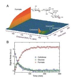
Fig. 6 Real-time observation of the conversion. Reaction conditions: 0.05 M [1'-13C] cellobiose, 0.6 M LiOH and 24 equiv. hydrogen peroxide in a 3 mm NMR tube (200 µL H<sub>2</sub>O/D<sub>2</sub>O (90%/10%)) at 308 K without agitation.
