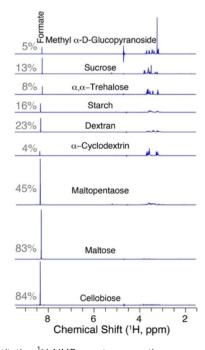
Fig. 5 Quantitative <sup>1</sup>H NMR spectra upon the conversion of various substrates under identical conditions, showing lower, but detectable, formate yields from non-reducing carbohydrates (grey fractions to the left). Reaction conditions: a concentration corresponding to 0.1 M glucose monomer, 0.6 M LiOH and 24 equiv. hydrogen peroxide in a 1.5 mL Eppendorf tube (200  $\mu$ L H<sub>2</sub>O/D<sub>2</sub>O (90%/10%)) at 308 K, shaken at 600 rpm for 20 h.
