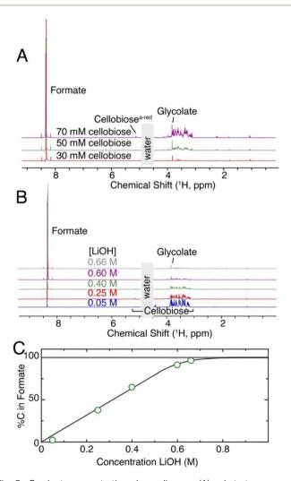
Fig. 3 Product concentration depending on (A) substrate concentration and (B and C) LiOH concentration. The line in (C) is a guide to the eye, and 0.6 M LiOH corresponds to 1 equiv. per substrate carbon. Reaction conditions: (A) variable and (B and C) 0.05 M cellobiose, (A) 0.6 M and (B and C) variable LiOH as indicated and 24 equiv. hydrogen peroxide in a 1.5 mL Eppendorf tube (200  $\mu$ L H<sub>2</sub>O/D<sub>2</sub>O (90%/10%)) at 308 K, shaken at 600 rpm for 20 h.
