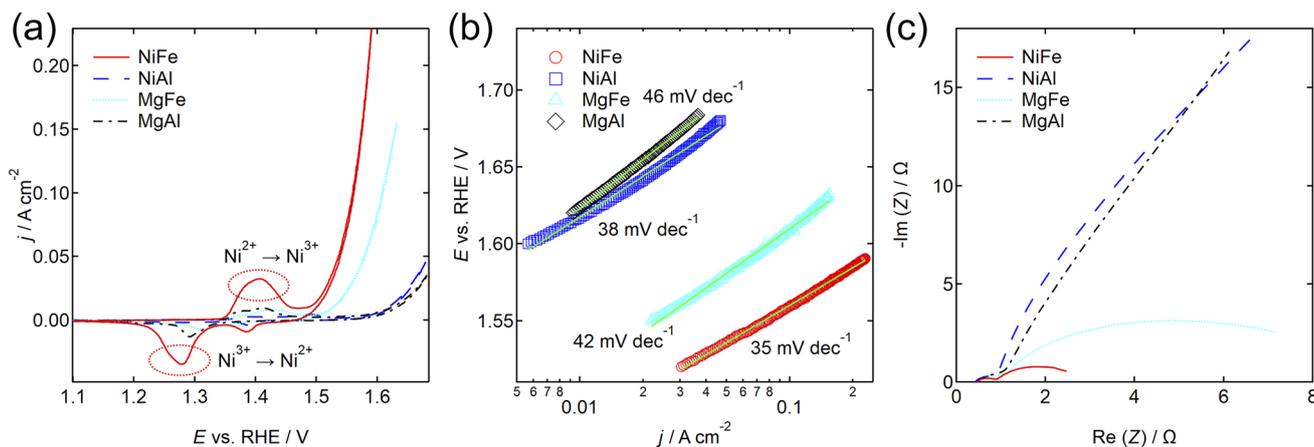
Fig. 2 (a) Cyclic voltammograms (CVs), (b) Tafel plots, and (c) Nyquist plots of NiFe-LDH/NF, NiAl-LDH/NF, MgFe-LDH/NF, and MgAl-LDH/NF in O<sub>2</sub>-saturated 1 mol dm<sup>-3</sup> KOH. The scans were performed at a scan rate of 5 mV<sup>-1</sup> in (a) and (b).
