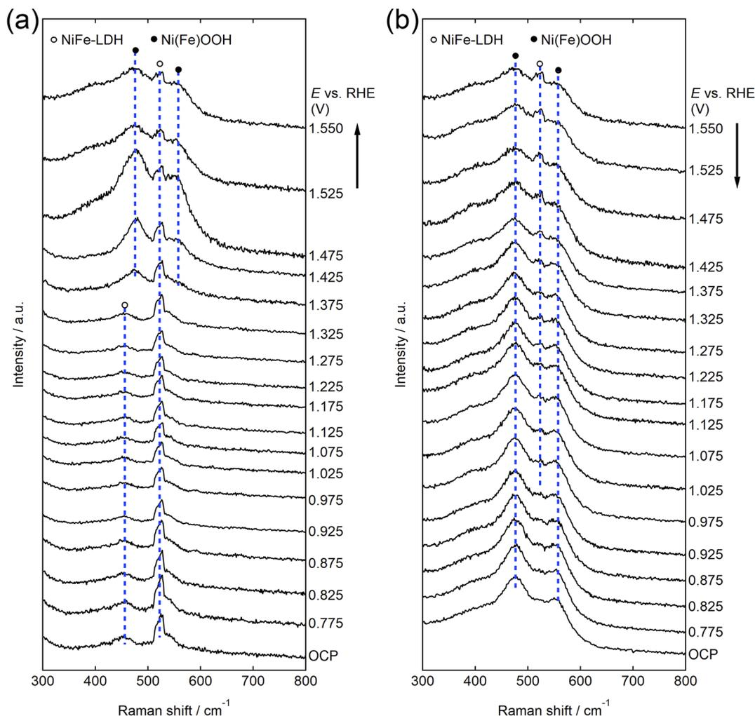
Fig. 4 *In situ* visible Raman spectra of a NiFe-LDH/Ni rod during (a) an increase in  $E$  from open circuit potential (OCP) to 1.550 V and (b) a decrease in  $E$  from 1.550 V to OCP in  $O_2$ -saturated  $1 \text{ mol dm}^{-3}$  KOH.
