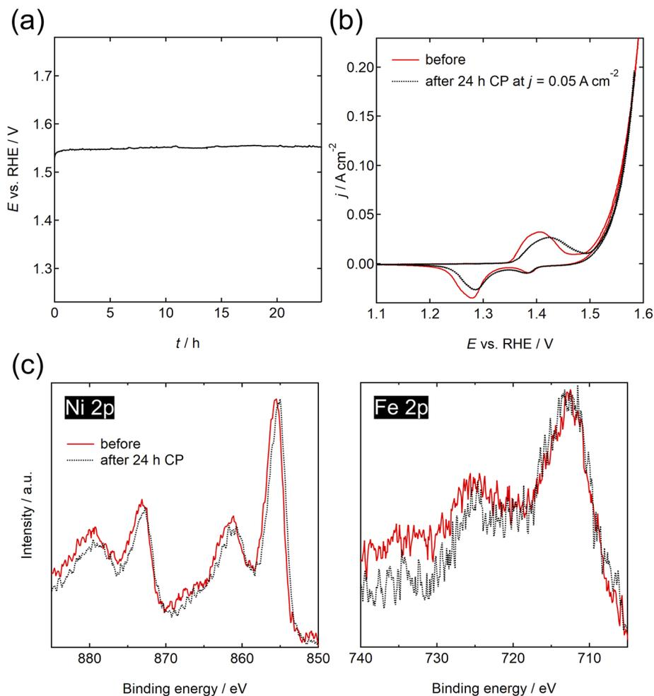
Fig. 3 (a) Potential versus time ( $E-t$ ) curve of NiFe-LDH/NF during chronopotentiometry (CP) at a constant current density,  $j = 0.05 \text{ A cm}^{-2}$ . (b) CV plots, (c) XP Ni 2p and Fe 2p spectra of NiFe-LDH/NF before (solid curves) and after (dashed curves) 24 h of CP at  $j = 0.05 \text{ A cm}^{-2}$ .
