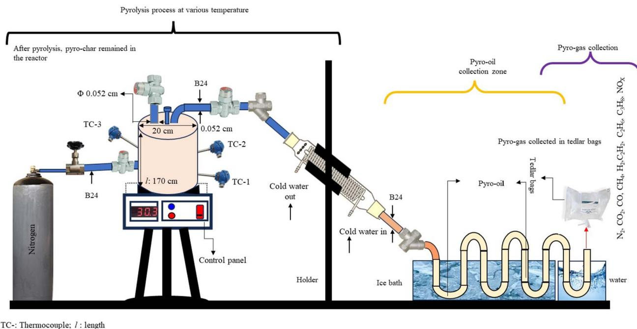
Fig. 2 Experimental setup used for the pyrolysis process.
