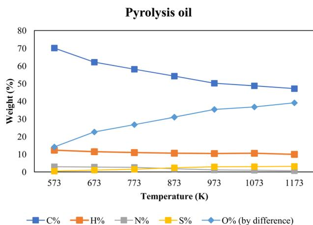
Fig. 11 Effect of CHNSO composition on pyrolysis oil.
