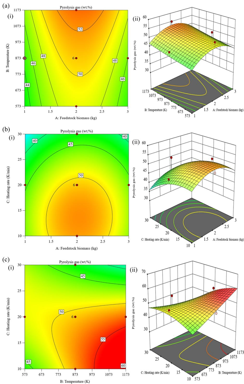
**Fig. 8** (a) (i) Two-dimensional contour and (ii) three-dimensional contour plots showing pyrolysis gas yield (wt%) as a function of feedstock biomass and temperature. (b) (i) Two-dimensional contour and (ii) three-dimensional contour plots showing pyrolysis gas yield (wt%) as a function of feedstock biomass and heating rate. (c) (i) Two-dimensional contour and (ii) three-dimensional contour plots showing pyrolysis gas yield (wt%) as a function of heating rate and temperature.
