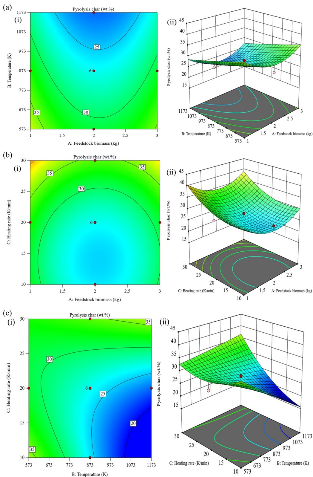
**Fig. 6** (a) (i) Two-dimensional contour and (ii) three-dimensional contour plots showing pyrolysis char yield (wt%) as a function of feedstock biomass and temperature. (b) (i) Two-dimensional contour and (ii) three-dimensional contour plots showing pyrolysis char yield (wt%) as a function of feedstock biomass and heating rate. (c) (i) Two-dimensional contour and (ii) three-dimensional contour plots showing pyrolysis char yield (wt%) as a function of heating rate and temperature.
