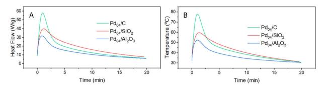
Fig. 1 TGA/DSC of  $Pd_{04}/C$ ,  $Pd_{04}/SiO_2$  and  $Pd_{04}/Al_2O_3$ . Catalysts (7.5 mg) were exposed to  $H_2$  at 10 mL min<sup>-1</sup> for 20 min with no additional external heating. Shown is heat flow in  $W g^{-1}$  (A) and temperature (B) to elucidate the heat generated by intrinsic and spontaneous Pd-hydride formation.
