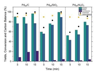
Fig. 2 Toluene, phenol and cyclohexanol yields, BPE conversion and overall carbon balance (%) with respect to increasing reaction time (5–15 min, 3 Hz) at 30 sccm  $H_2$ . For each experiment, 0.2 g of BPE was used in combination with 0.25 g of catalyst.
