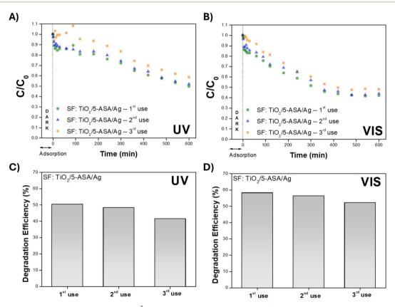
Fig. 6 Photocatalytic degradation of CIP ( $C_0 = 5 \text{ mg L}^{-1}$ ) in three consecutive uses of SF: TiO<sub>2</sub>/5-ASA/Ag membranes irradiated for 600 min with (A) UV, (B) VIS and their respective degradation efficiency (%) in (C) and (D).
