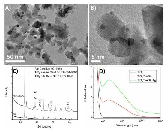
Fig. 2 (a) Low- and (b) high-magnification TEM images of  $TiO_2/5$ -ASA/Ag nanocomposites. (c) XRD of  $TiO_2/5$ -ASA/Ag nanocomposites. (d) Kubelka–Munk transformation of reflection spectra of commercial  $TiO_2$  and synthesised  $TiO_2/5$ -ASA and  $TiO_2/5$ -ASA/Ag nanocomposites.
