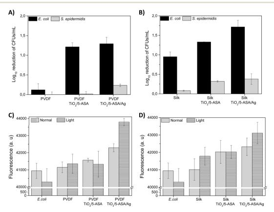
Fig. 7 . Antibacterial activity of (A) PVDF-HFP-based membranes and (B) SF-based membranes in terms of *E. coli* and *S. epidermidis* log<sub>10</sub> reduction, and dichlorofluorescein fluorescence intensity in *E. coli* in contact with (C) PVDF-HFP-based membranes and (D) SF-based membranes, in "normal" conditions and after application of the sun-mimicking light.
