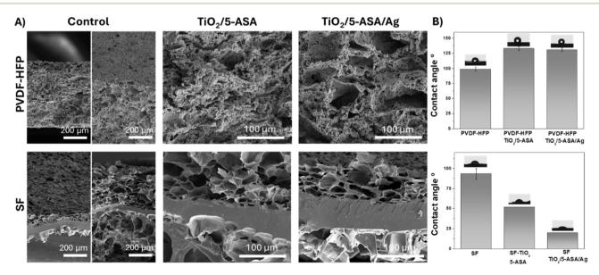
Fig. 3 (A) Cross-sectional and tilted SEM images of porous membranes composed of PVDF-HFP and SF with TiO<sub>2</sub>/5-ASA and TiO<sub>2</sub>/5-ASA/Ag fillers. SEM images of controls are at  $250 \times$  magnification, while fillers are at  $1000 \times$  magnification. (B) Contact angle of the different membranes.
