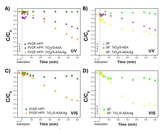
Fig. 5 Photocatalytic degradation of CIP ( $C_0 = 5 \text{ mg L}^{-1}$ ) with (A) PVDF-HFP and (B) SF-based membranes over 600 min of UV irradiation; with (C) PVDF-HFP and (D) SF-based membranes over 600 min of VIS irradiation.
