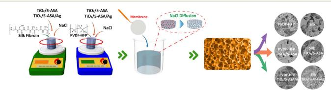
Fig. 1 Schematic representation of the methodology to develop the PVDF-HFP- and SF-based pristine and nanocomposite membranes.
