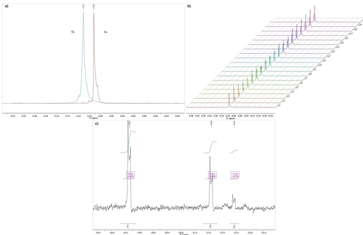
Fig. 5 (a) Reference <sup>1</sup>H NMR spectra of D<sub>4</sub> and D<sub>6</sub> in acetone-*d*<sub>6</sub>, (b) <sup>1</sup>H NMR array experiment following the rearrangement (1 : 10) of D<sub>6</sub> over 50 minutes at -5 °C, (c) <sup>29</sup>Si NMR spectrum of the products of this rearrangement showing D<sub>4</sub> (A), D<sub>5</sub> (B) and D<sub>6</sub> (C).
