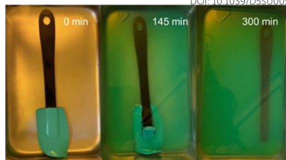
Figure 2. Images taken throughout the depolymerization of a silicone spatula in methyl ethyl ketone (MEK) and 1 mol% TBAF. The silicone head is dissolved while the plastic handle remains unaffected.
