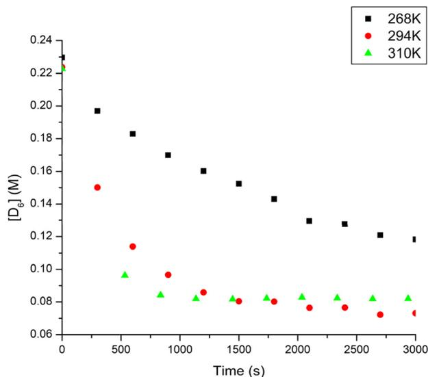
Fig. 6 The depletion of  $D_6$  siloxane over time due to fluoride-induced rearrangement.
