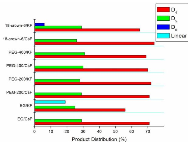
Fig. 7 Smooth-Sil 950 depolymerization products in MEK as determined by  $^{29}\text{Si}$  NMR. (Fig. S62–S69†).
