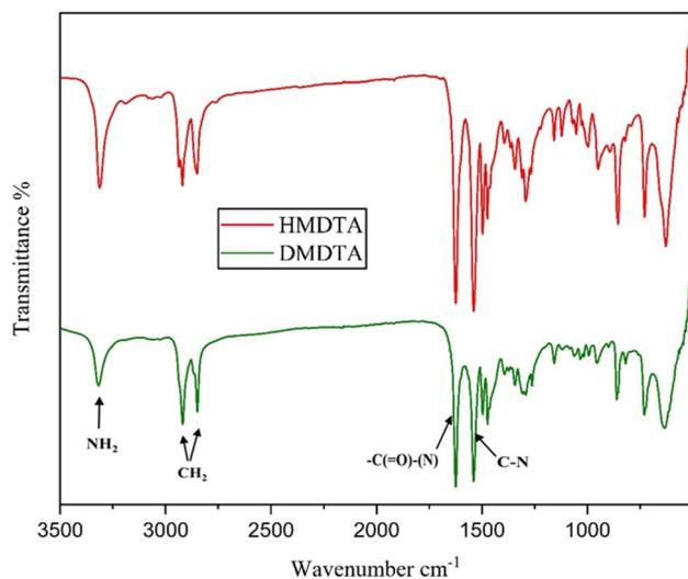
Fig. 3 FTIR spectrum of recovered terephthalamides.
