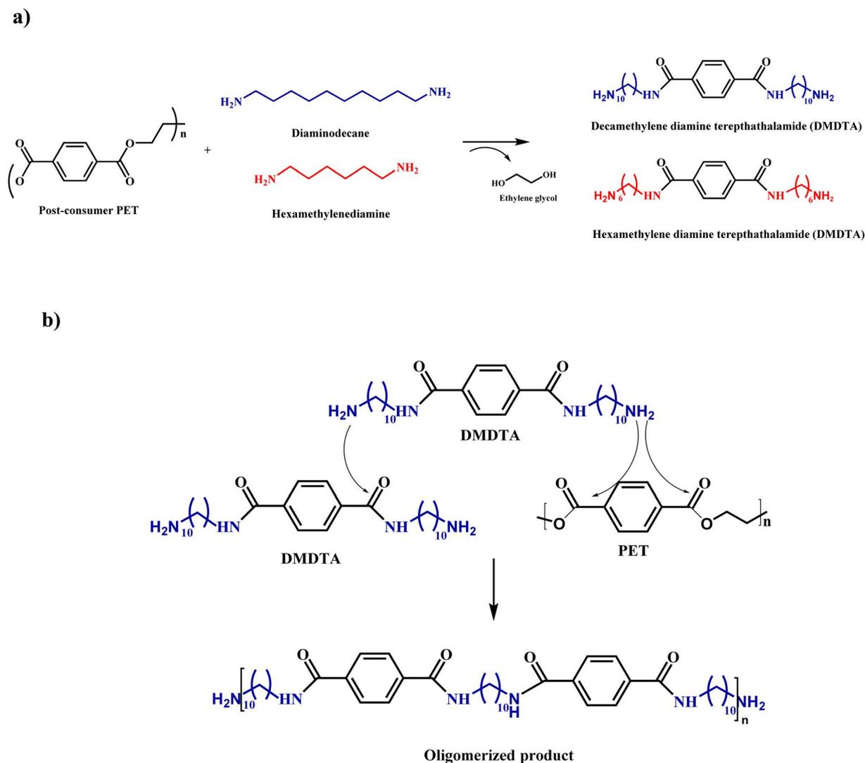
Fig. 1 (a) Aminolysis reaction scheme of PET into terephthalamides, (b) side reactions associated with oligomerization during aminolysis.
