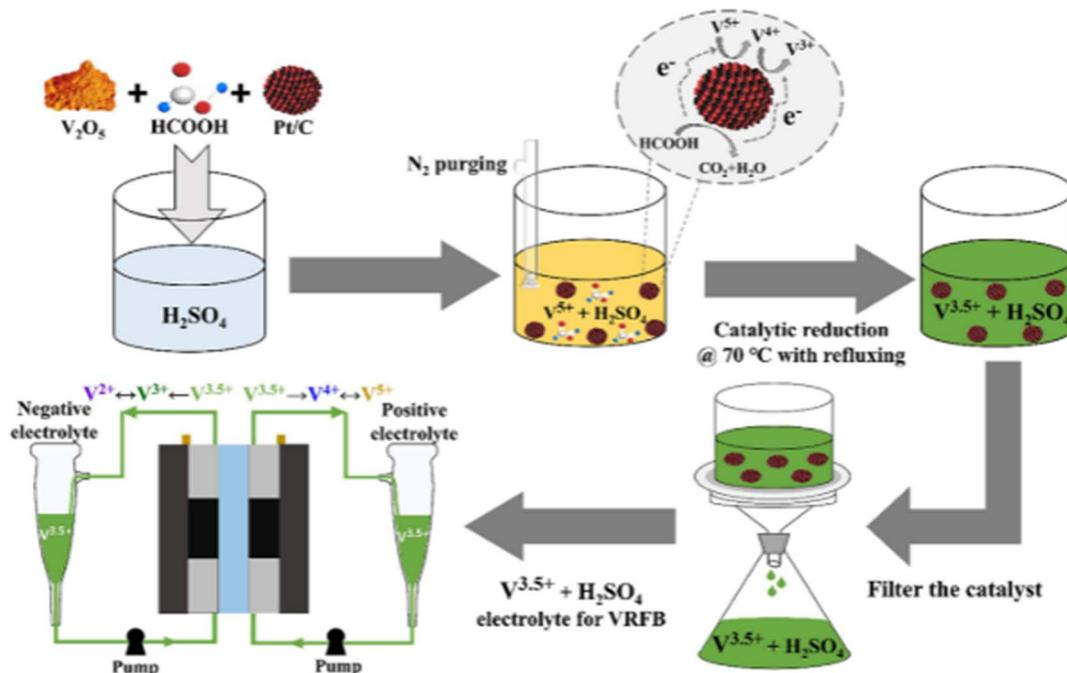
Fig. 8 Schematic of  $V^{3.5+}$  electrolyte preparation using hydrothermal reduction<sup>16</sup> (reprinted with permission from American Chemical Society).
