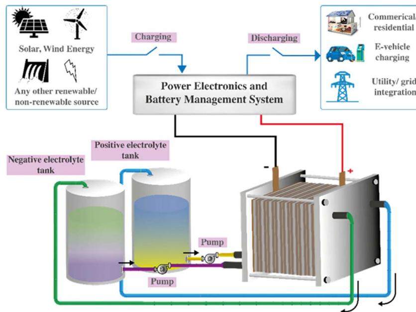
Fig. 1 VFB energy storage schematic<sup>15</sup> (reprinted with permission from Springer Nature).
