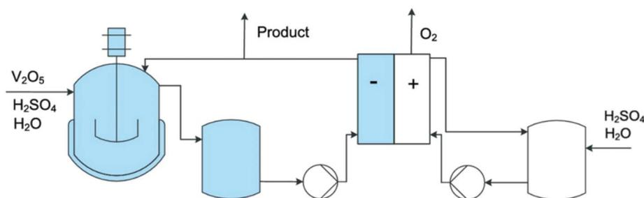
Fig. 16 Process flow for production of vanadium electrolyte<sup>72</sup> (reprinted with permission from John Wiley and Sons).
