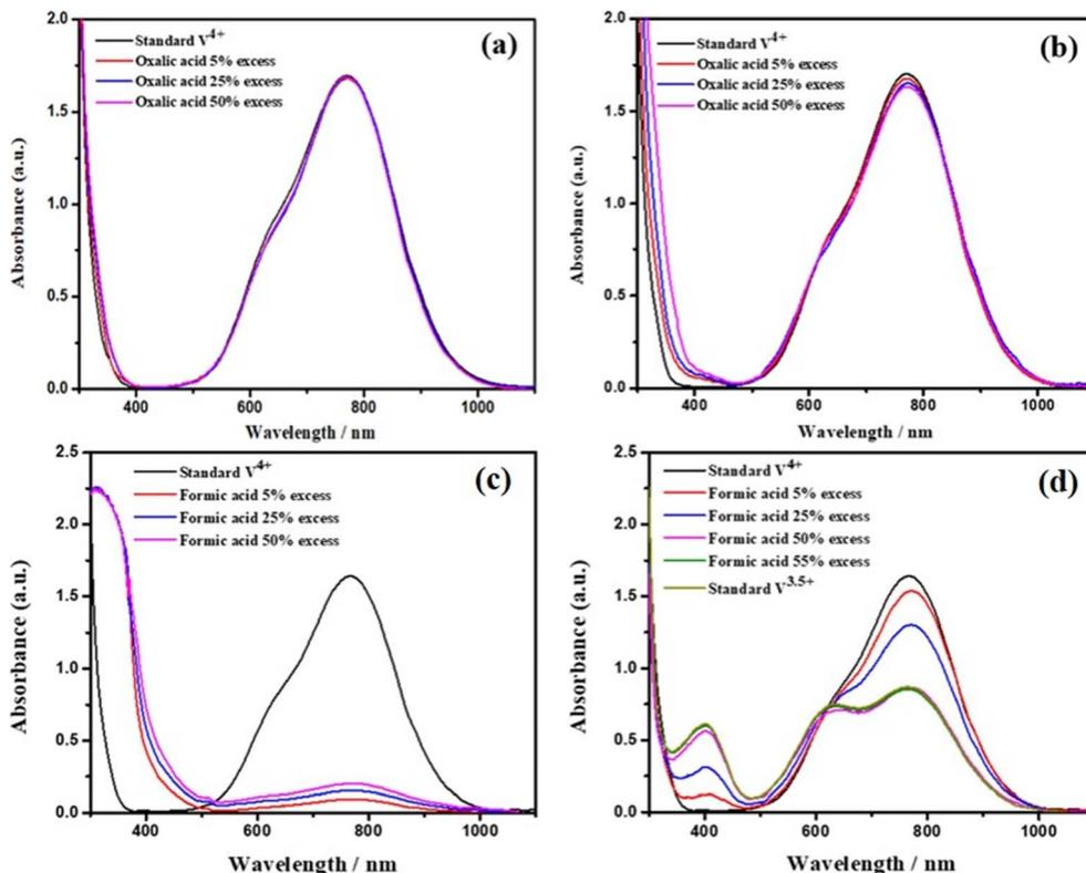
Fig. 9 UV-vis spectra of the electrolyte with (a) oxalic acid; (b) oxalic acid in the presence of a Pt/C catalyst; (c) formic acid; (d) formic acid in the presence of a Pt/C catalyst<sup>16</sup> (reprinted with permission from American Chemical Society).
