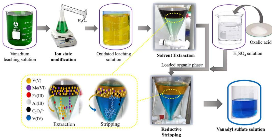
Fig. 19 Flow diagram of a solvent extraction–complexation reduction–stripping method<sup>87</sup> (reprinted with permission from Elsevier).
