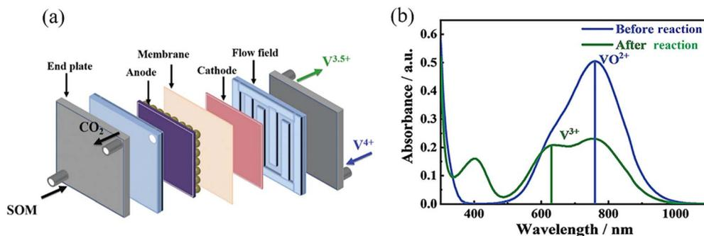
Fig. 13 (a) Schematic diagram and reaction mechanism of the fuel cell reactor; (b) UV-vis spectra of the electrolytes before and after the reaction<sup>52</sup> (reprinted with permission from MDPI).
