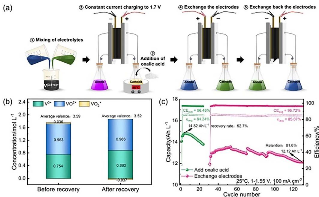
Fig. 22 (a) Schematic diagram; (b) comparison of electrolyte composition; (c) discharge specific capacity.<sup>111</sup>
