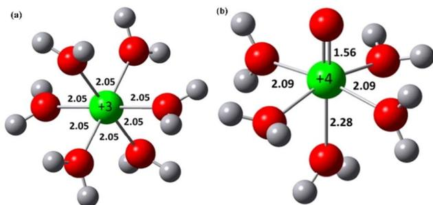
Fig. 3 Structures of (a)  $V^{3+}$  and (b)  $V^{4+}$  ions and their first solvation shell water molecules by DFT<sup>44</sup> (reprinted with permission from Elsevier).
