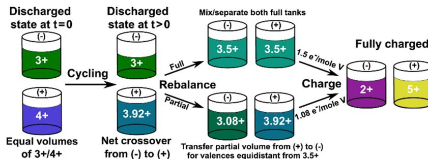
Fig. 21 Schematic of the full and partial rebalancing techniques<sup>26</sup> (reprinted with permission from Elsevier).
