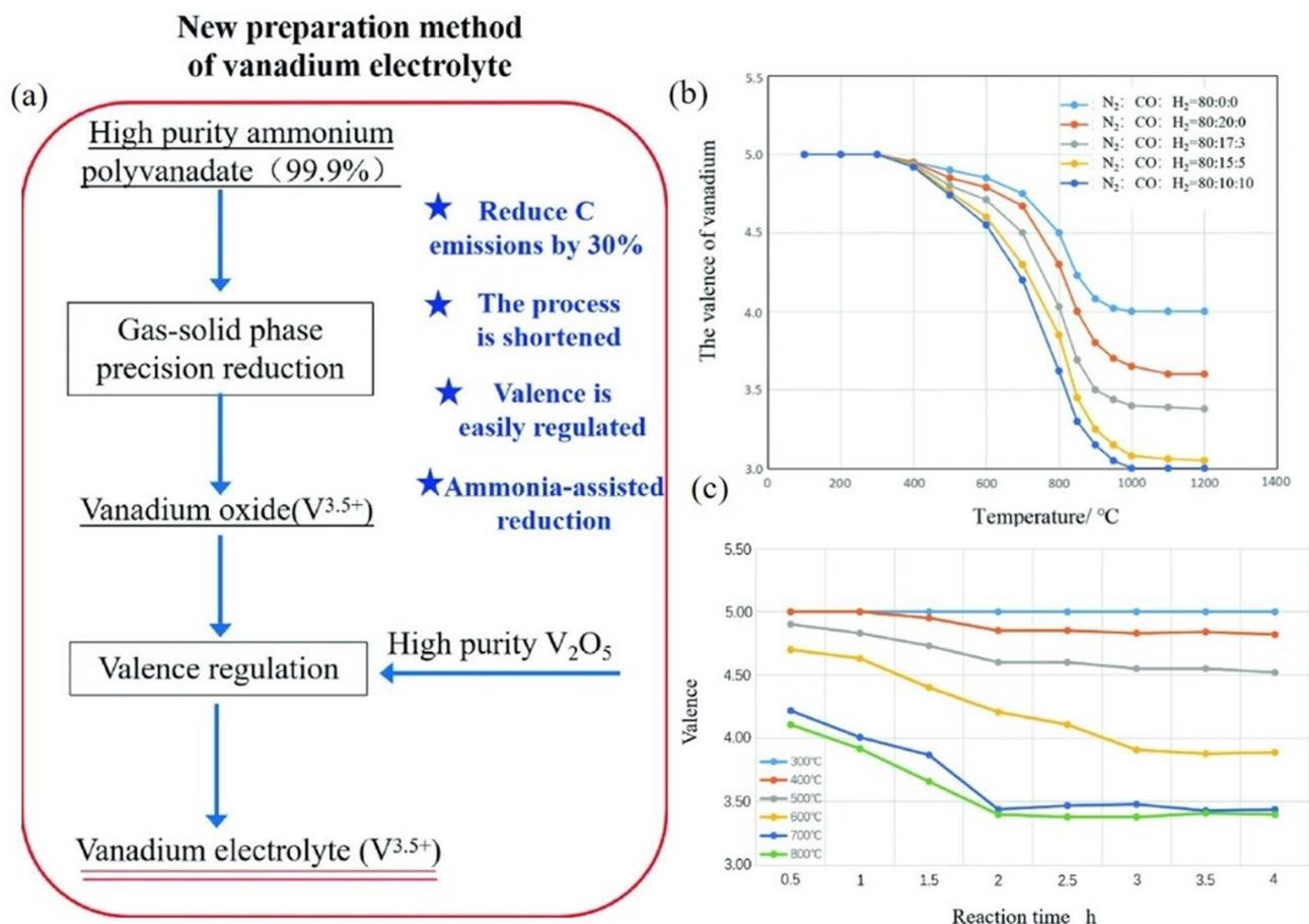
Fig. 6 (a) Process flow; the influence of (b) different reducing agent partial pressures; (c) temperature and reduction time<sup>66</sup> (reprinted with permission from Springer Nature).
