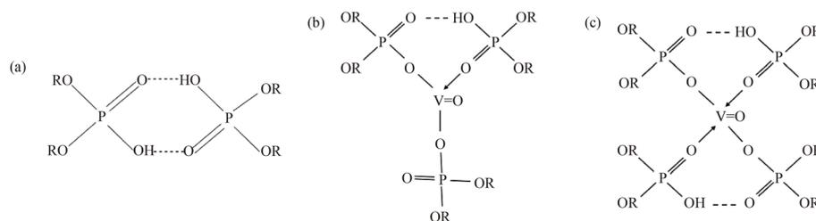
Fig. 18 (a) Dimer structure of the D2EHPA extractant in the organic phase; (b and c) VO<sup>2+</sup> ions coordinate with multiple D2EHPA monomers in the loaded organic phase<sup>84</sup> (reprinted with permission from Springer Nature).
