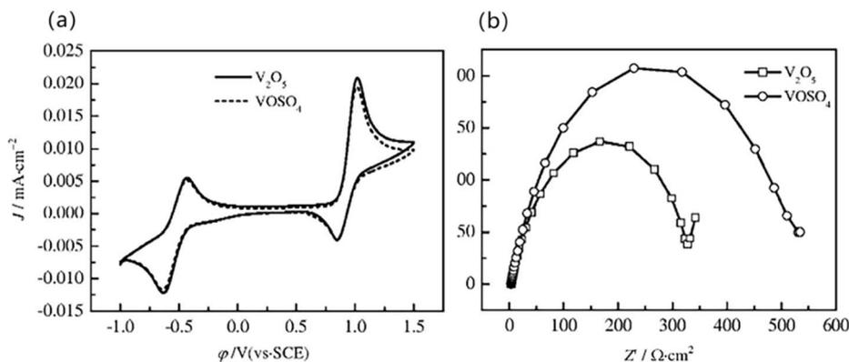
Fig. 5 (a) CV; (b) impedance spectrum of  $V^{3+}$  electrolytes prepared with different raw materials<sup>59</sup> (reprinted with permission from MDPI).
