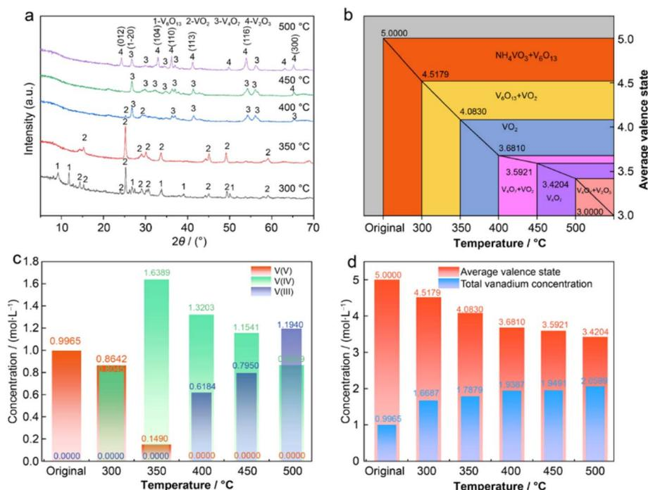
Fig. 7 At different temperatures: (a) XRD; (b) the average valence state and phase change; (c) the concentration of vanadium; (d) the variation of total vanadium concentration and average valence state<sup>67</sup> (reprinted with permission from Springer Nature).
