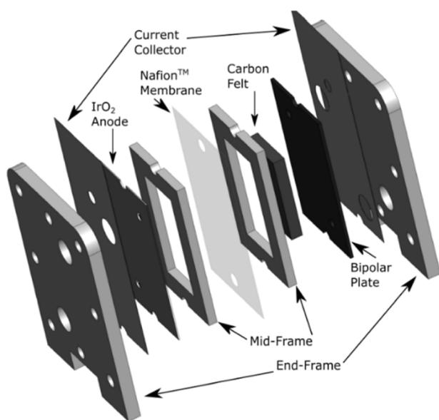
Fig. 14 Schematic diagram of the battery structure used in oxygen evolution electrolysis<sup>72</sup> (reprinted with permission from John Wiley and Sons).
