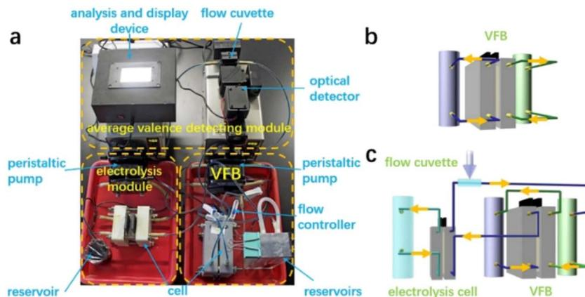
Fig. 23 (a) The photo capacity recovery system (b) in the normal mode and (c) in the recovery mode<sup>114</sup> (reprinted with permission from Elsevier).
