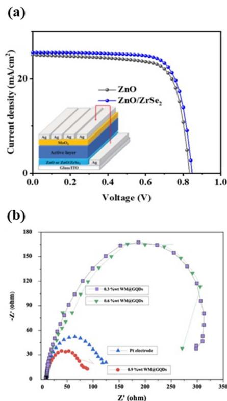
Fig. 6 (a)  $J$ - $V$  curves of OSCs with PM6:L8-BO as the active layer and different ETLs measured at AM 1.5G irradiation (inset: schematic of the OSC). Reproduced from ref. 97 with permission from Wiley-VCH Verlag GmbH & Co., copyright 2024. (b) Electrochemical impedance spectroscopy profiles of different counter electrodes for DSSCs. Reproduced from ref. 98 with permission from Springer Nature, copyright 2023.
