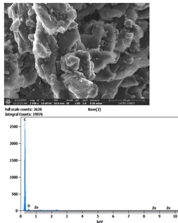
Fig. 4 SEM coupled with EDX analysis of bio-NPs-ZnO/CPE.
