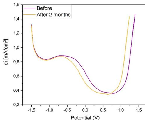
Fig. 13 Bio-NPs-ZnO/CPE stability; amplitude: 20 mV; potential step: 5 mV; start potential:  $-1.5$  V vs. Hg/Hg<sub>2</sub>Cl<sub>2</sub>, KCl sat.
