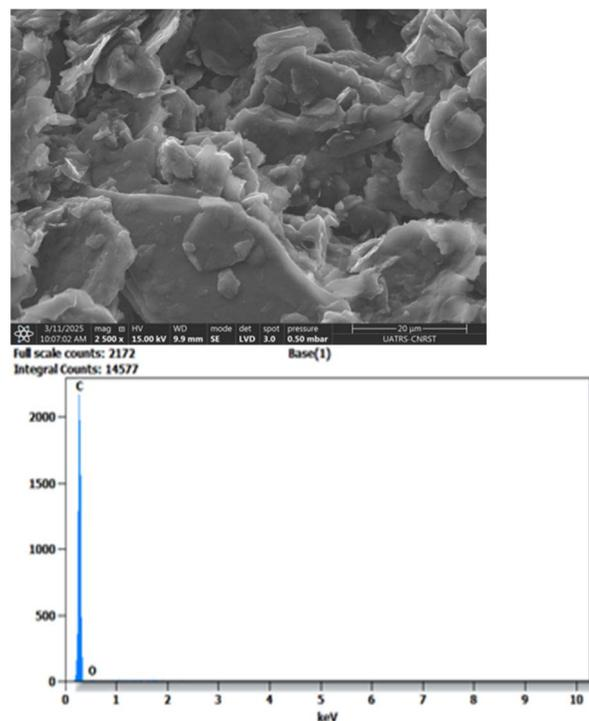
Fig. 3 SEM coupled with EDX analysis of CPE.
