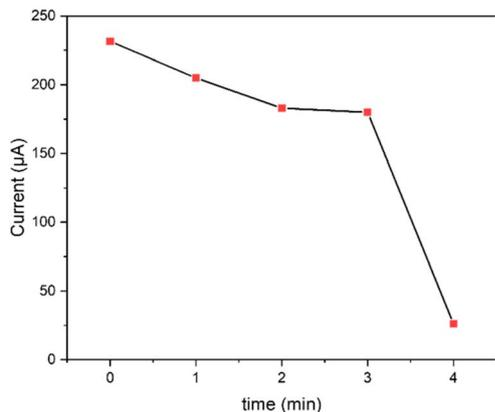
Fig. 9 Effect of accumulation time on the peak current of totarolone at the bio-NPs-ZnO/CPE electrode in 0.1 M NaCl solution (pH 4.5), at a scan rate of  $100 \text{ mV s}^{-1}$  and a start potential of  $-1.0 \text{ V vs. Hg/Hg}_2\text{Cl}_2, \text{KCl}_{\text{sat}}$ .
