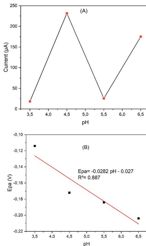
Fig. 8 (A) Influence of solution pH on the oxidation peak current of totalolone recorded at bio-NPs-ZnO/CPE in 0.1 M NaCl, at a scan rate of 100 mV s<sup>-1</sup> and a start potential of  $-1.0$  V *vs.* Hg/Hg<sub>2</sub>Cl<sub>2</sub>, KCl sat, and (B) linear plot of  $E_{pa}$  *vs.* pH.
