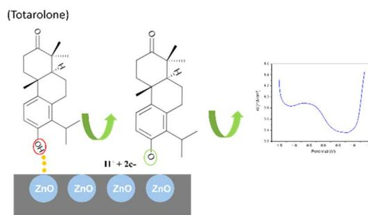
Fig. 14 Proposed mechanism of totarolone detection on bio-NPs-ZnO/CPE.
