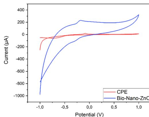
Fig. 6 CV measurements for both the CPE and bio-NPs-ZnO/CPE in 2 mM totarolone dissolved in 0.1 M NaCl, at a scan rate of  $100 \text{ mV s}^{-1}$  and a start potential of  $-1.0 \text{ V}$  vs.  $\text{Hg}/\text{Hg}_2\text{Cl}_2$ ,  $\text{KCl}/\text{sat}$ .
