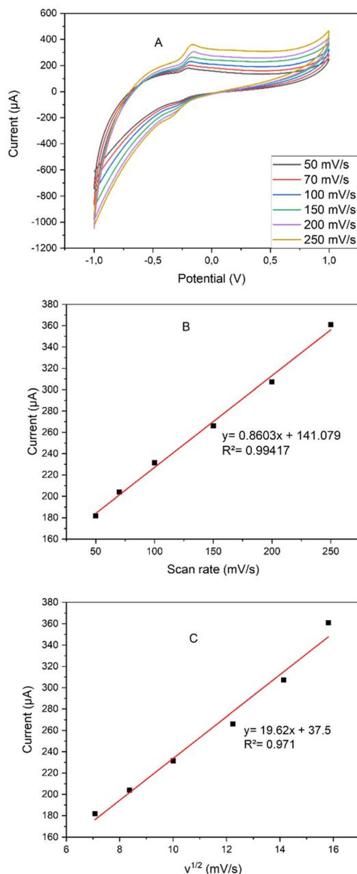
Fig. 7 (A) Bio-NPs-ZnO/CPE CVs in 0.1 M NaCl solution (pH = 4.5) with 2 mM of totalolone at various SRs and a start potential of  $-1.0$  V *vs.* Hg/Hg<sub>2</sub>Cl<sub>2</sub>, KCl sat. (B) Plot of  $I_{pa}$  *versus*  $v$ . (C) Plot of  $I_{pa}$  *versus*  $v^{1/2}$ .
