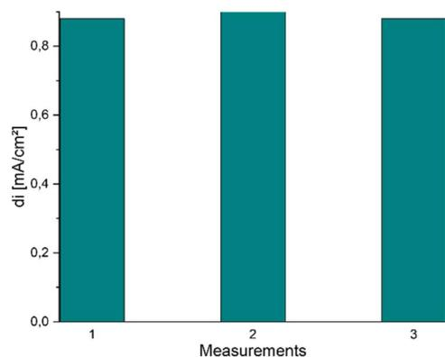
Fig. 12 Evaluation of the reproducibility of bio-NPs-ZnO/CPE; amplitude: 20 mV; potential step: 5 mV; start potential:  $-1.5$  V vs. Hg/Hg<sub>2</sub>Cl<sub>2</sub>, KCl sat.
