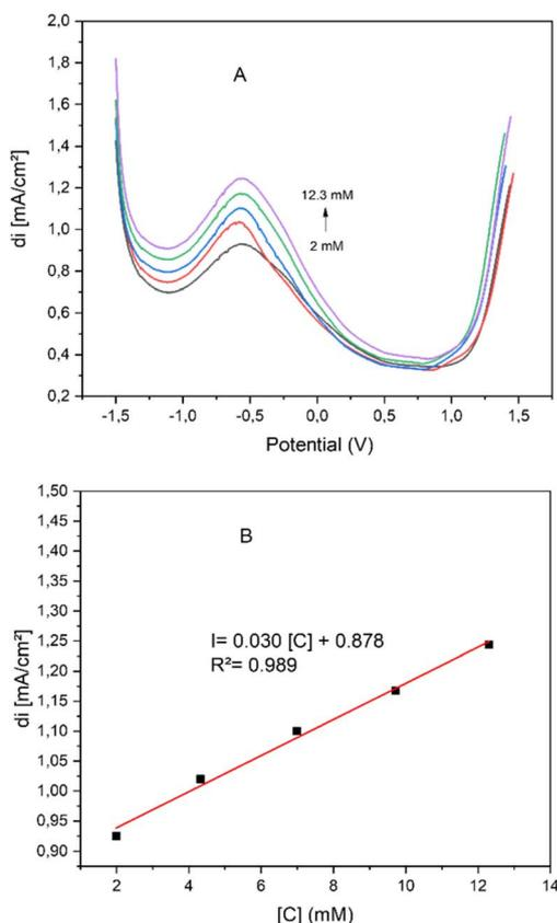
Fig. 10 (A) SW voltammograms of bio-NPs-ZnO/CPE for the determination of totarolone in 0.1 M NaCl solution (pH 4.5); amplitude: 20 mV; potential step: 5 mV; start potential:  $-1.5 \text{ V vs. Hg/Hg}_2\text{Cl}_2, \text{KCl}_{\text{sat}}$ . (B) Calibration graph corresponding to the peak of totarolone obtained from various concentrations in the range of 2 to 12.3 mM.
