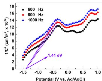
Fig. 9 UV-vis absorption spectrum of T(4-COOH)PP (a) and its derivatives (b and c), XPS valence band of T(4-COOH)PP (d), and Mott-Schottky curves of T(4-COOH)PP (e).
