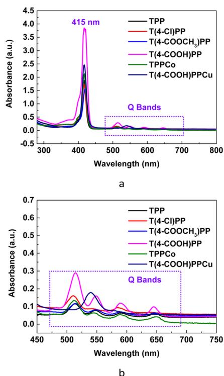
Fig. 1 UV-vis absorption spectra of representative porphyrins and metalloporphyrins in DMF ( $4 \times 10^{-6}$  mol L<sup>-1</sup>) (a) and their Q bands (b).
