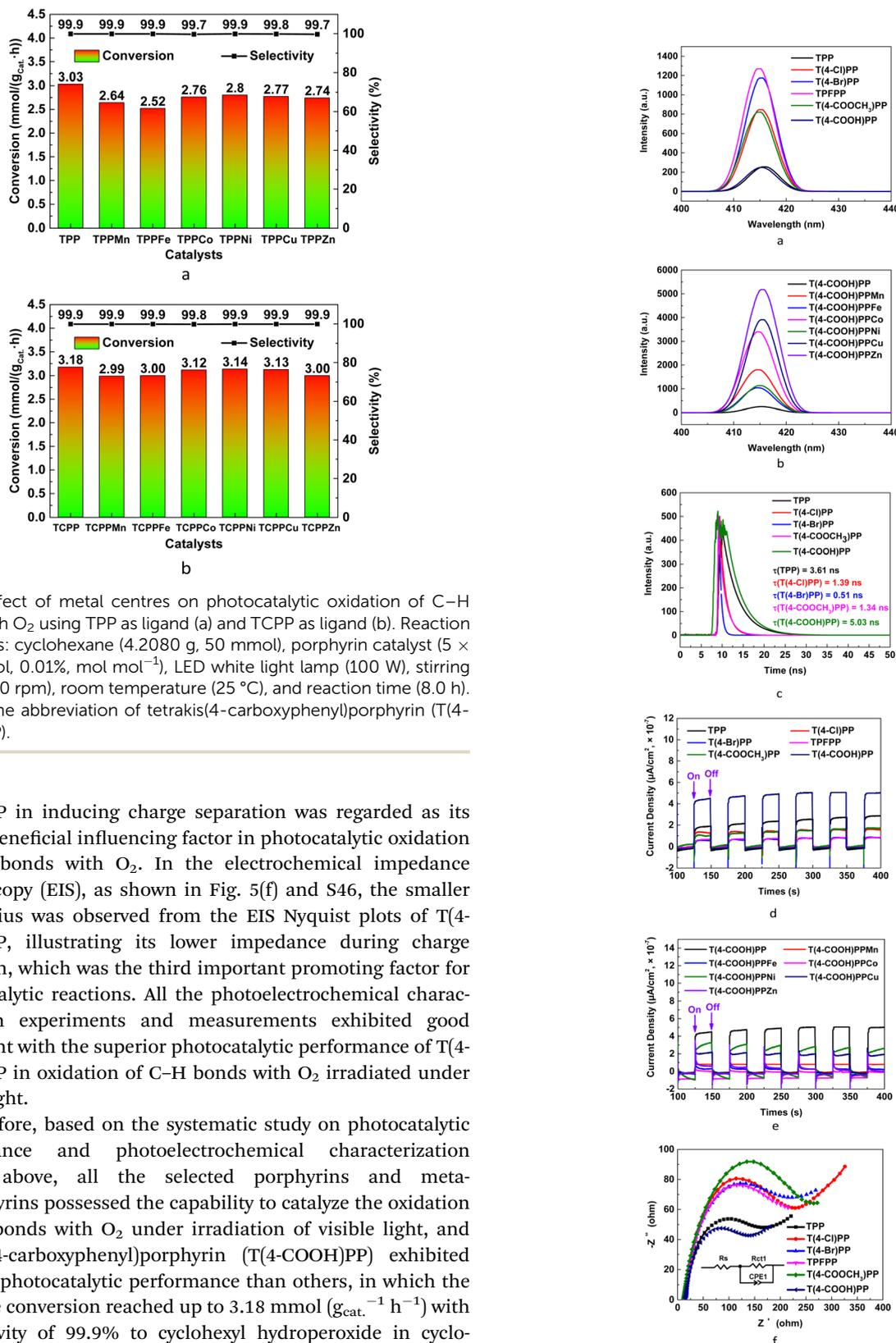
Fig. 4 Effect of metal centres on photocatalytic oxidation of C–H bonds with O<sub>2</sub> using TPP as ligand (a) and TCPP as ligand (b). Reaction conditions: cyclohexane (4.2080 g, 50 mmol), porphyrin catalyst (5 × 10<sup>-3</sup> mmol, 0.01%, mol mol<sup>-1</sup>), LED white light lamp (100 W), stirring speed (600 rpm), room temperature (25 °C), and reaction time (8.0 h). TCPP is the abbreviation of tetrakis(4-carboxyphenyl)porphyrin (T(4-COOH)PP).
