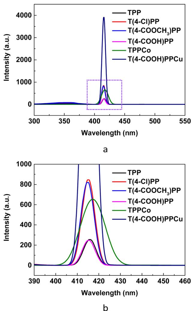
Fig. 2 PL emission spectra of representative porphyrins and metalloporphyrins in DMF (a), and local magnification (b) ( $4 \times 10^{-6}$  mol L<sup>-1</sup>).
