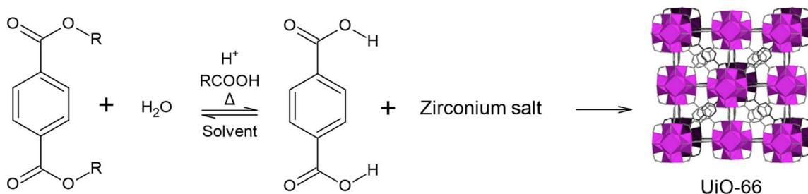
Scheme 1 Proposed one-pot synthetic route of UiO-66 starting from a terephthalate diester (R =  $-\text{CH}_3$  or  $-\text{CH}_2\text{CH}_2\text{OH}$ ).
