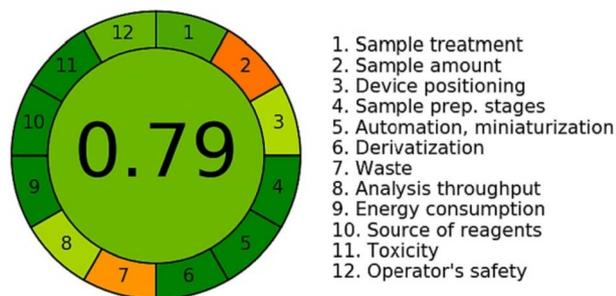
Fig. 23 Greenness assessment of the developed voltammetric method with a sustainable sensor strip employing AGREE metric assessment tool. Source: reproduced with permission from Raymundo-Pereira *et al.* (2023) *Biomater. Adv.*<sup>96</sup>
