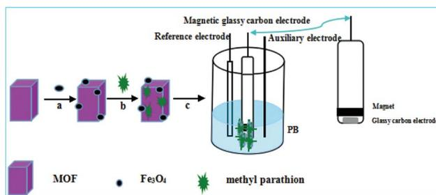
Fig. 24 Schematic representation of  $\text{Fe}_3\text{O}_4$ /MOF synthesis. Source: reproduced with permission from Hu *et al.* (2014) *Anal. Sci.*<sup>97</sup>
