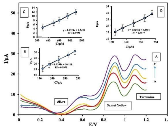
Fig. 21 DPV of  $\text{IL}/\text{NiFe}_2\text{O}_4/\text{rGO}/\text{CPE}$  in pH 3 with varying concentrations of Allura Red, Sunset Yellow, and Tartrazine DPVs; insets: linear ranges for Allura Red (B), Sunset Yellow (C), and Tartrazine (D). Source: reproduced with permission from Darabi *et al.* (2021).<sup>85</sup> Copyright Food Chem.
