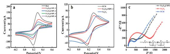
Fig. 18 Cyclic voltammograms of various modified electrodes in (a and b) 5 mm Fe(CN)<sub>6</sub><sup>3-/4-</sup> redox probe containing 0.1 M KCl. (c) Nyquist plots of PCM/GCE, Fe<sub>3</sub>O<sub>4</sub>@MPC-2/GCE and Fe<sub>3</sub>O<sub>4</sub>. Source: reproduced with permission from Liu *et al.* (2022).<sup>72</sup> Copyright *Adv. Mater. Interfaces*.
