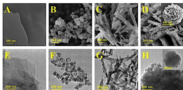
Fig. 20 SEM (A–D) and TEM (E–H) images of EG (A and E),  $p\text{-Fe}_2\text{O}_3$  (B and F),  $r\text{-Fe}_2\text{O}_3$  (C and G) and  $f\text{-Fe}_2\text{O}_3$  (D and H). The insets in (D) and (H) show the low-magnification SEM and TEM images, respectively. Source: reproduced with permission from Chen *et al.* (2019).<sup>84</sup>
