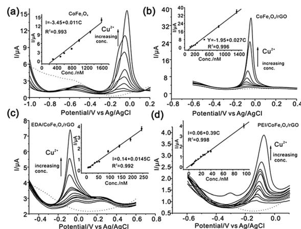
Fig. 13 Typical SWASV responses of (a) CoFe<sub>2</sub>O<sub>4</sub>, (b) CoFe<sub>2</sub>O<sub>4</sub>/rGO, (c) EDA/CoFe<sub>2</sub>O<sub>4</sub>/rGO, and (d) PEI/CoFe<sub>2</sub>O<sub>4</sub>/rGO. Source: reproduced with permission from Xiong *et al.* (2016).<sup>69</sup> Copyright *Electrochim. Acta*.
