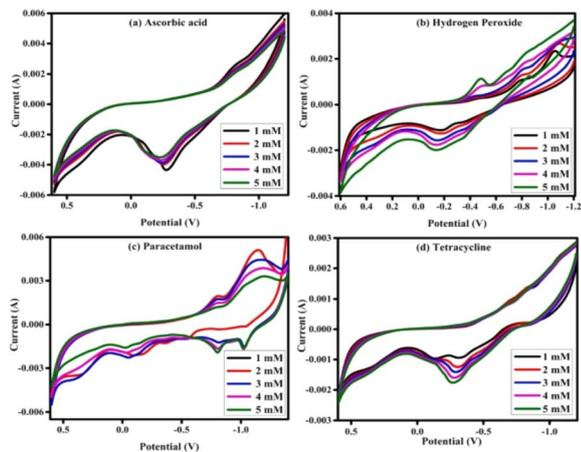
Fig. 27 Cyclic voltammograms of  $\text{Fe}_3\text{O}_4\text{-MoS}_2$  for the detection of (a) AA (b) HP (c) PCM and (d) TC. N Source: reproduced with permission from Halligudra *et al.* (2022).<sup>100</sup> Copyright *Ceram. Int.*
