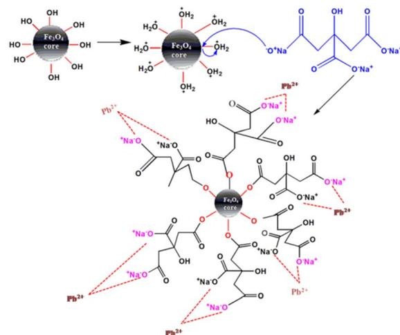
Fig. 6 Mechanistic illustration of removal of positively charged heavy metal ions by citrate-coated magnetite nanoparticles.
