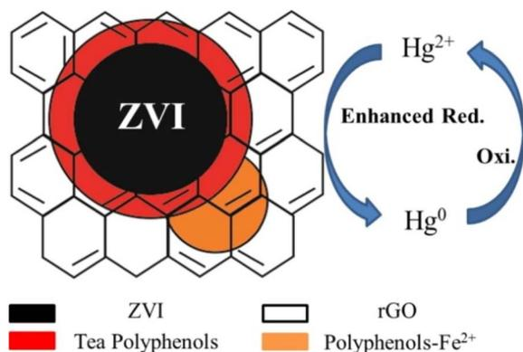
Fig. 7 Role of zerovalent iron in the removal of inorganic and organic contaminants from aqueous systems. Source: reproduced with permission from Bao et al. (2022).<sup>54</sup> Copyright *J. Electroanal. Chem.*
