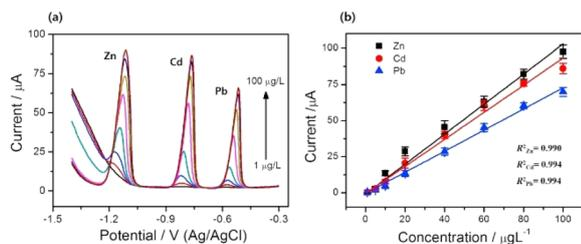
Fig. 15 (a) Stripping voltammograms for varied Zn<sup>2+</sup>, Cd<sup>2+</sup>, and Pb<sup>2+</sup> ion concentrations on the Fe<sub>2</sub>O<sub>3</sub>/G/Bi composite film electrode. (b) Calibration plot for the detection of Zn<sup>2+</sup>, Cd<sup>2+</sup>, and Pb<sup>2+</sup>. Source: reported with permission from Lee *et al.* (2016), *Talanta*.<sup>71</sup>
