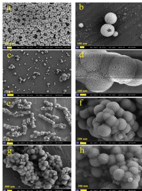
Fig. 17 SEM images of (a) Fe<sub>3</sub>O<sub>4</sub>, (b and c) Fe<sub>3</sub>O<sub>4</sub>@MPC-1, (d and e) Fe<sub>3</sub>O<sub>4</sub>@MPC-2, (f and g) Fe<sub>3</sub>O<sub>4</sub>@MPC-3, and (h) Fe<sub>3</sub>O<sub>4</sub>@MPC-4. Source: reproduced with permission from Liu *et al.* (2022).<sup>72</sup> Copyright *Adv. Mater. Interfaces*.
