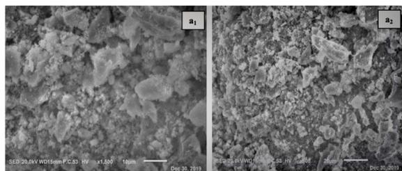
Fig. 12 SEM images (a<sub>1</sub> and a<sub>2</sub>) of the Fe<sub>2</sub>O<sub>3</sub>@Ni/Al-LDH sample. Source: reproduced with permission from Dib *et al.* (2021).<sup>68</sup> Copyright *Inorg. Chem. Commun.*
