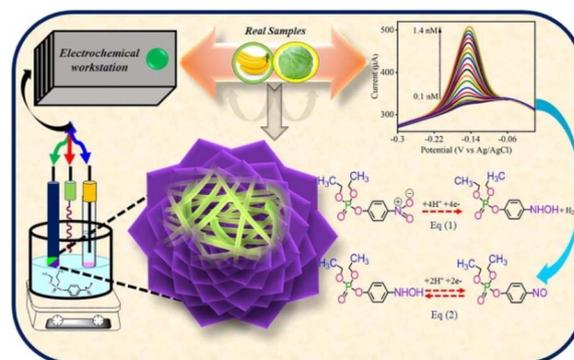
Fig. 25 Synthesis of  $\text{NiCo}_2\text{O}_4$ -SWCNT composites for the detection of paraoxon ethyl. Reproduced with permission from Kulkarni *et al.* (2023) *J. Electroanal. Chem.*<sup>98</sup>
