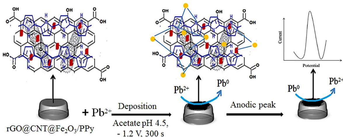
Fig. 10 Detection of  $\text{Pb}^{2+}$  ions on the surface of  $\text{rGO@CNT@Fe}_2\text{O}_3/\text{PPy}$  electrode. Source: reproduced with permission from Fall *et al.* (2021)<sup>65</sup> *Mater. Today Commun.*
