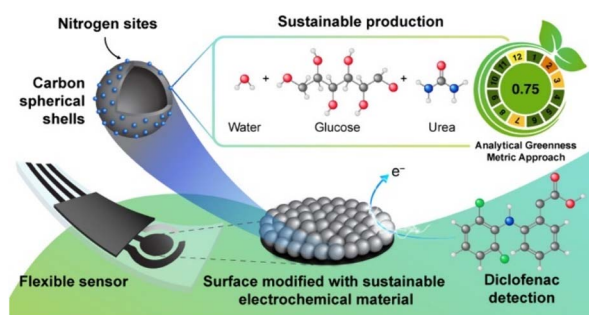
Fig. 28 Electrochemical quantification of diclofenac using N-CSSs. Source: reproduced with permission from Raymundo-Pereira et al. (2024). 101 Copyright ACS Appl. Nano Mater.
