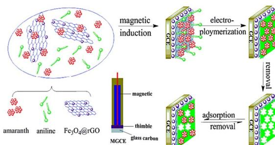
Fig. 22 Figure illustrating the process of creating a  $\text{Fe}_3\text{O}_4/\text{rGO}$  doped molecularly imprinted polymer membrane that uses a magnetic field to detect amaranth. Source: reproduced with permission from Han *et al.* (2014).<sup>86</sup> Copyright Talanta.
