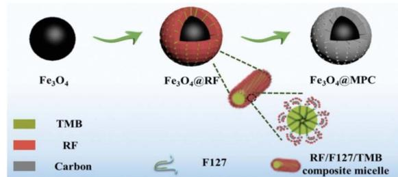
Fig. 16 Mechanism of preparation of magnetic Fe<sub>3</sub>O<sub>4</sub>@MPC core-shell nanospheres. Source: reproduced with permission from Liu *et al.* (2022).<sup>72</sup> Copyright *Adv. Mater. Interfaces*.
