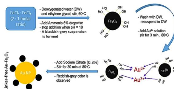
**Fig. 11** Diagram illustrating the synthesis and proposed formation mechanism of  $\text{Fe}_3\text{O}_4\text{-Au}$  nanoparticles. Source: reproduced with permission from Sedki *et al.* (2021)<sup>67</sup> *Sensors*.
