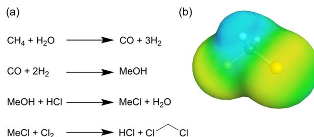
Fig. 1 (a) Four stage synthesis of methylene chloride from methane via methanol. (b) COSMO surface of methylene chloride indicating positive charge in blue, neutral charge in green and negative charge in yellow.
