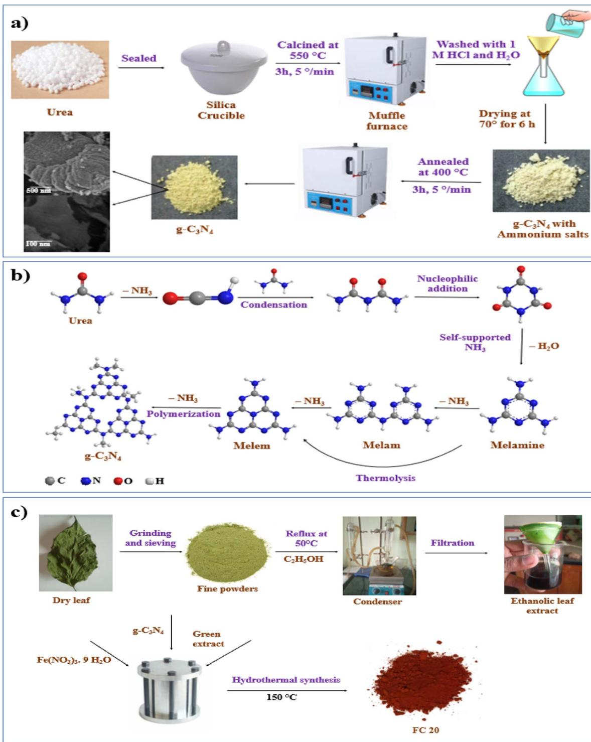
Scheme 1 Graphical representation of catalyst fabrication. (a) Preparation of  $g\text{-C}_3\text{N}_4$ ; (b) mechanism of  $g\text{-C}_3\text{N}_4$  formation; (c) preparation of  $\alpha\text{-Fe}_2\text{O}_3/g\text{-C}_3\text{N}_4$  heterojunction.
