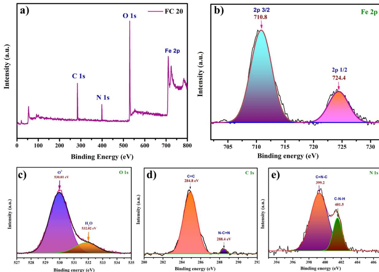
Fig. 5 XPS survey of FC 20 (a), and high-resolution binding spectra of Fe 2p (b), O 1s (c), C 1s (d), and N 1s (e).
