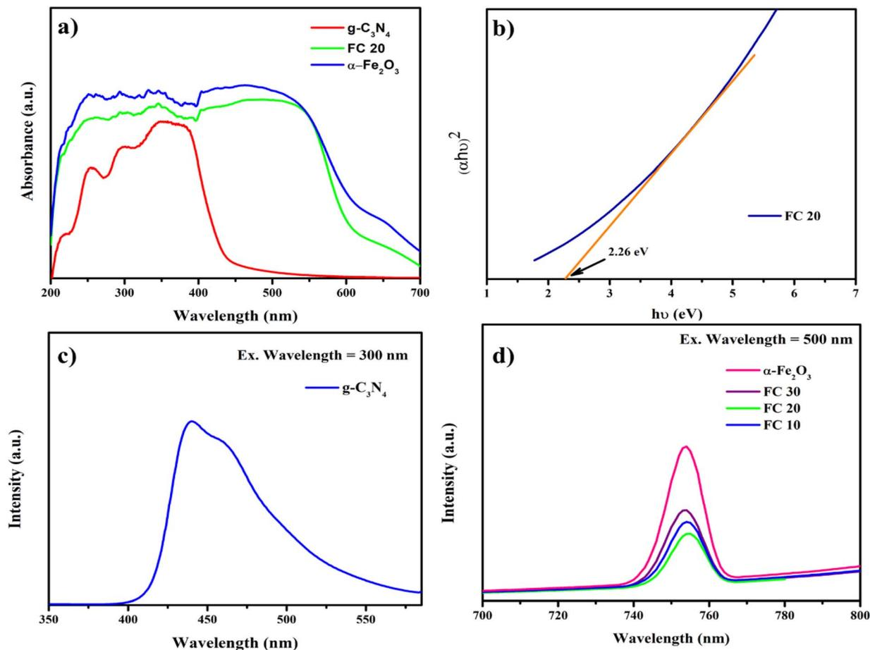
Fig. 6 UV-Vis DRS spectra of  $\alpha$ -Fe<sub>2</sub>O<sub>3</sub>, g-C<sub>3</sub>N<sub>4</sub>, and FC 20 (a), Tauc plot of FC 20 (b), and PL spectra of g-C<sub>3</sub>N<sub>4</sub> (c),  $\alpha$ -Fe<sub>2</sub>O<sub>3</sub> and heterostructures (d).
