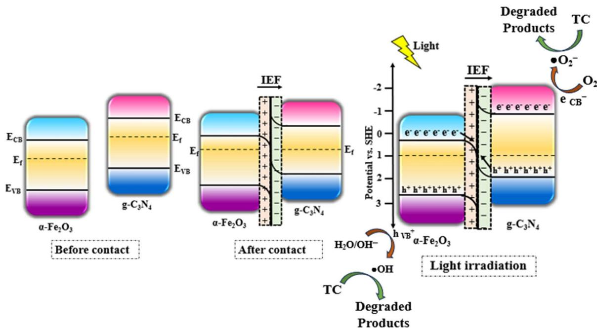
Scheme 3 Proposed S-scheme charge transfer mechanism in  $\alpha\text{-Fe}_2\text{O}_3/\text{g-C}_3\text{N}_4$ .
