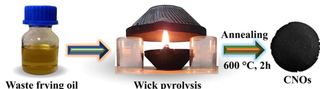
Fig. 6 A schematic illustration for the synthesis of CNOs by the flame pyrolysis method. 77
