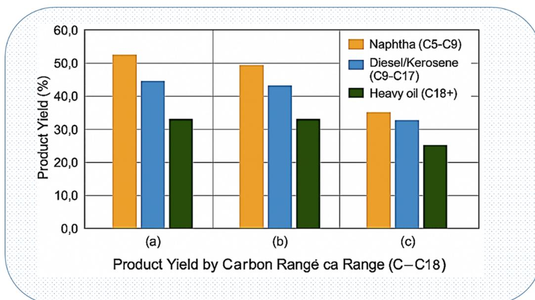
Fig. 7 Yield of pyrolysis for oil fractions by carbon range (C5 to C18).
